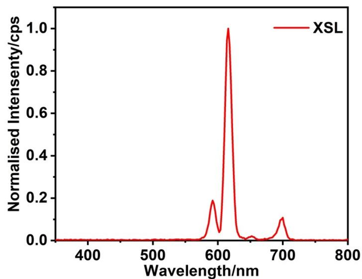
**Figure S9.** Solid-state XSL (a high-purity tungsten target with a tube voltage of 50 kV and a tube current of 100  $\mu$ A) spectra of **PMOF-2** at room temperature.
