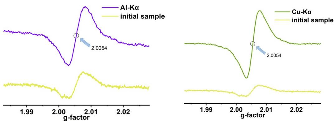
**Figure S7.** EPR signals of the Al-K $\alpha$  and Cu-K $\alpha$  X-ray irradiated samples for compound **PMOF-2**.
