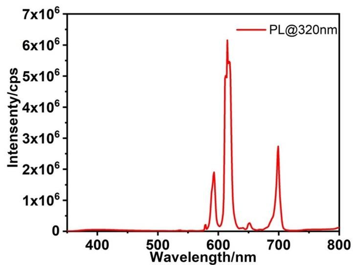
**Figure S8.** Solid-state photoluminescence (PL; excitation wavelength, 320 nm) spectra of **PMOF-2** at room temperature.
