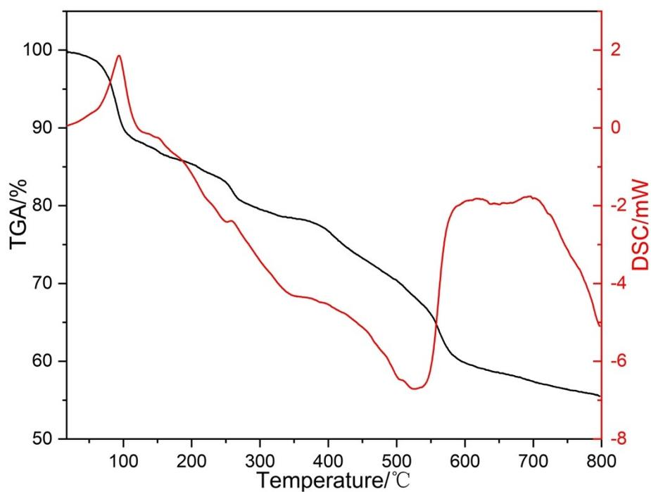
**Figure S11.** TGA and DSC curves of **PMOF-2**.
