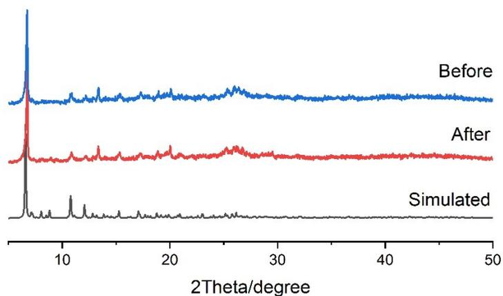
**Figure S6.** The PXRD patterns of **PMOF-2** simulated, before and after (Cu-K $\alpha$  X-ray) irradiation at 25°C.
