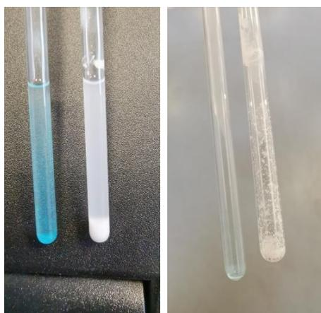
Figure S3. NMR tubes after depolymerization of blue and white PLA : left (deposit of the solid in the crude mixture), right : isolated solid
