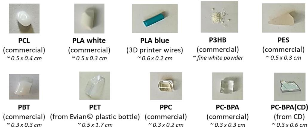
Figure S1. Commercial polymers and plastics depolymerized
