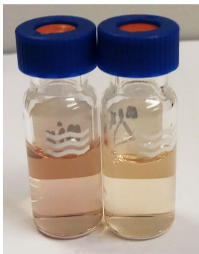
**Figure S14.** Visible colour change observed in 1:1 **DAN-NDI-DAN:NDI-DAN-NDI** at room temperature (left) and above 45 °C (right)
