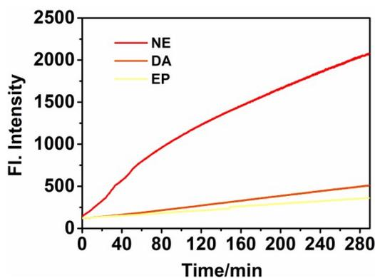
**Figure S6.** The time dependent of 20  $\mu\text{M}$  probe upon 5 mM NE, DA and EP in 0-300 min.
