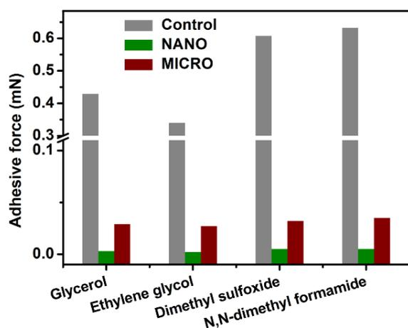
**Fig. S7** Plot of adhesive force of contacted glycerol, ethylene glycol, dimethyl sulfoxide and N,N-dimethyl formamide droplets. The values of adhesive forces were acquired
