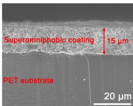
**Fig. S6** FE-SEM image of cross-sectional poc-F<sub>13</sub>POSS-wrapped SiO<sub>2</sub> nanoparticle-based coatings on a polyethylene terephthalate (PET) substrate.
