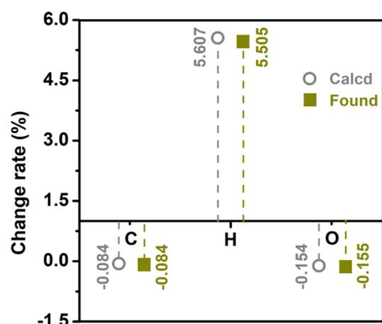
**Fig. S2** Plot of element change rate of poc-F<sub>13</sub>POSS-2OH<sub>2</sub><sup>+</sup> relative to poc-F<sub>13</sub>POSS-2OH.
