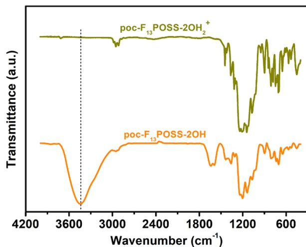
**Fig. S3** FTIR spectra of poc-F<sub>13</sub>POSS-2OH and poc-F<sub>13</sub>POSS-2OH<sub>2</sub><sup>+</sup>. In poc-F<sub>13</sub>POSS-2OH profile, a band at *ca.* 3420 cm<sup>-1</sup> was attributed to stretching vibration of Si-OH. In poc-F<sub>13</sub>POSS-2OH<sub>2</sub><sup>+</sup> profile, the band at 3420 cm<sup>-1</sup> disappeared, which was closely related with -OH protonation.
