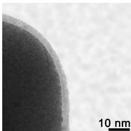
**Fig. S4** TEM image of poc-F<sub>13</sub>POSS-wrapped ZrO<sub>2</sub> nanoparticle.
