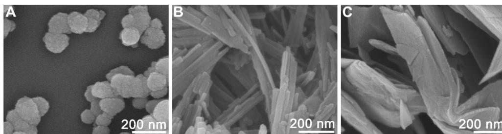
**Fig. S5** FE-SEM images of (A) ZrO<sub>2</sub> nanoparticles, (B) ATP nanorods and (C) GO nanosheets.
