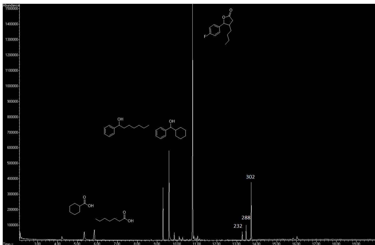
Figure S5: Gas chromatograms for 1-Hexene exchange reaction without lithium chloride. More pinacol coupling product (1,2-bis(4-fluorophenyl)ethane-1,2-diol) is formed instead which is not visible here and is very easy to separate. The numbers above the peaks are the mass for M^+ ion if the compound could not be identified.
