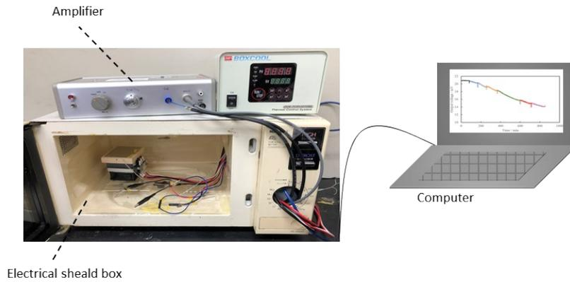
**Fig. S5** Detection system configuration.
