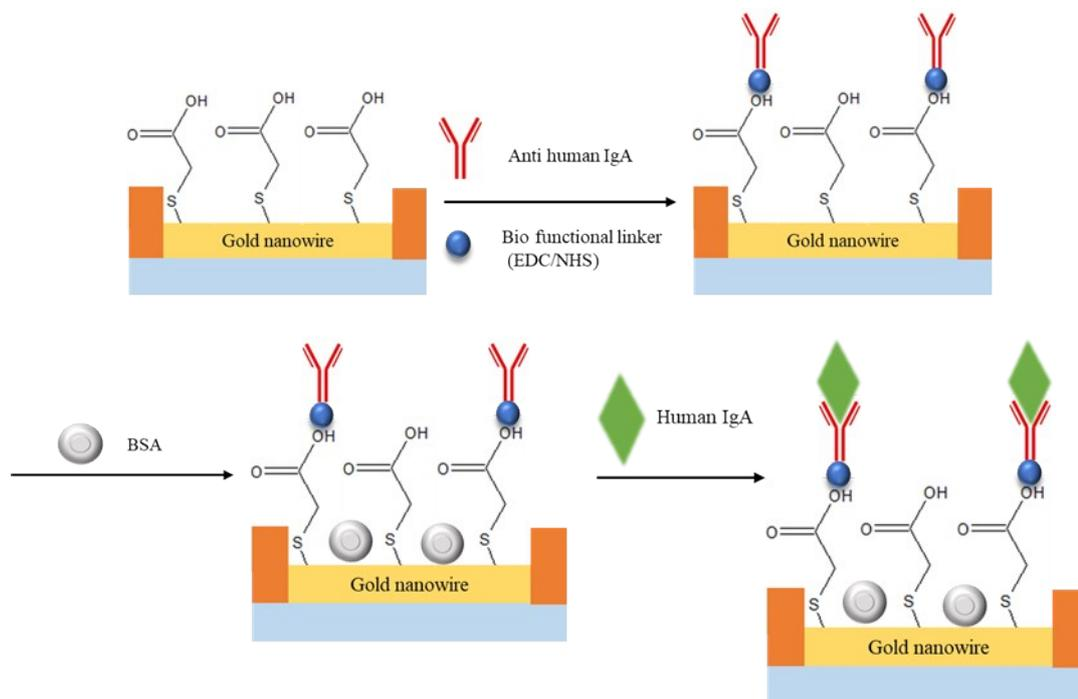
**Fig. S7** The scheme of the gold nanowire functionalization.
