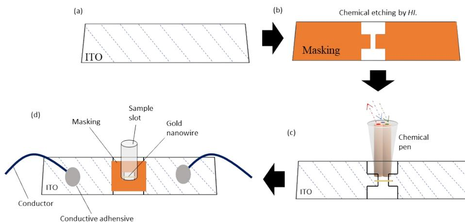
**Fig. S6** Scheme of fabricating biosensor. (a) ITO glass. (b) Masking of chemical etching. (c) Fabrication of the gold nanowire between ITO electrodes. (d) Installation of conductors and sample slot and protection of the gold nanowire.
