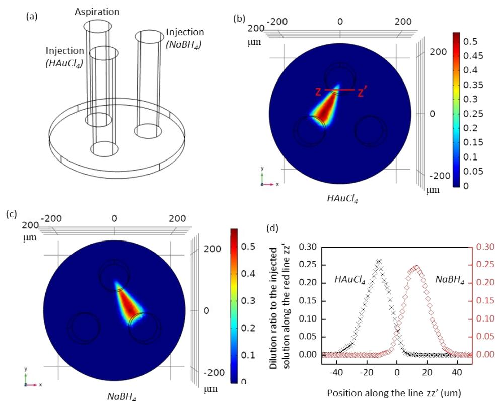
**Fig. S2** Calculated solution concentration at middle position between the substrate and the bottom surface of the chemical pen. (a) 3D model of chemical pen. (b) Concentration distribution of gold chloride. (c) Concentration distribution of sodium borohydride. (d) Dilution ratio to the injected solution along the red line  $zz'$  shown in Fig. S2b.
