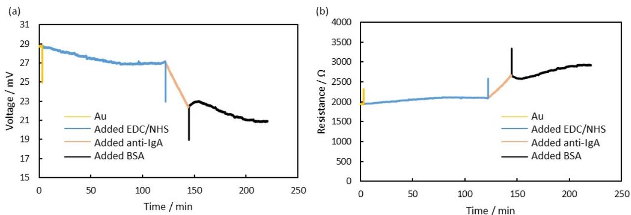
**Fig. S8** Real time measurement when functionalizing the gold nanowire. (a) Real time measurement of voltage. (b) Calculated resistance.
