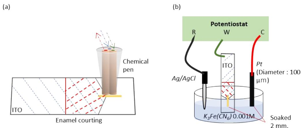
**Fig. S4** Scheme of CV measurement. (a) Fabrication of working electrode with chemical pen. (b) Scheme of CV measurement.
