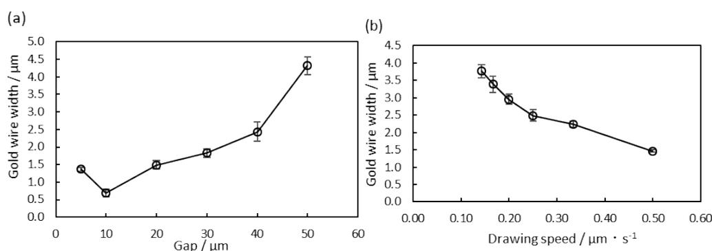
**Fig. S3** Width of gold wire in each condition as optimization results. (a) Gold wire width when gap was changed. (b) Gold wire width with various drawing speeds.
