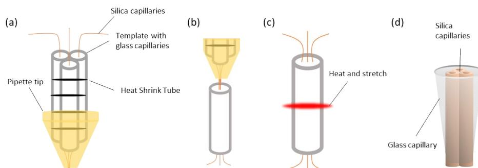
**Fig. S1** Brief fabrication method of the chemical pen. (a) Three silica capillaries were bundled using a template. (b) The bundled three silica capillaries were put through one glass capillary. (c) The glass capillary was heated and stretched to fold the silica capillaries. (d) Schematic diagram of the fabricated the chemical pen.
