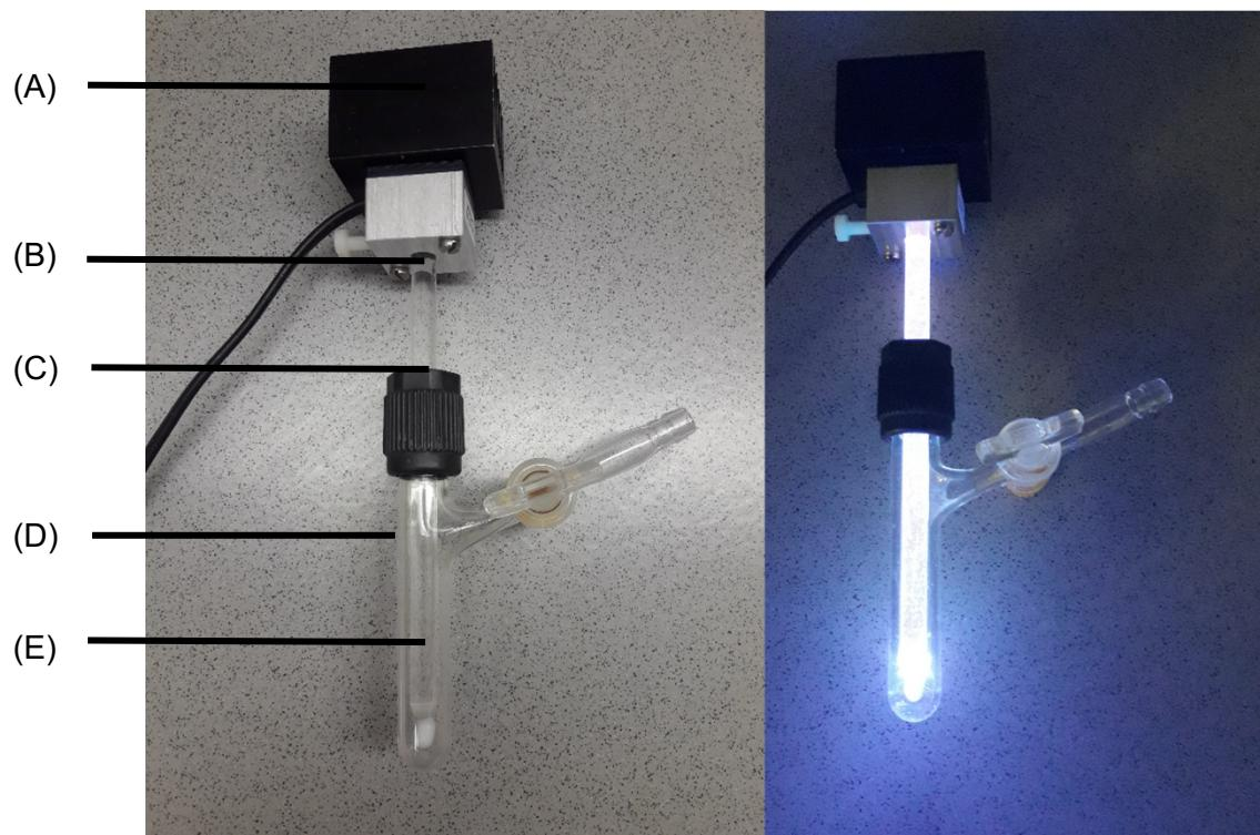
**Figure S1:** Irradiation setup for photochemical reactions: (A) LED; (B) glass rod; (C) Teflon adapter; (D) Schlenk tube (10.0 mL size); (E) Teflon-coated stirring bar.
