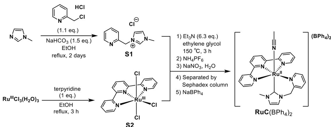
**Scheme S1.** Synthesis of **RuC(BPh<sub>4</sub>)<sub>2</sub>**.
