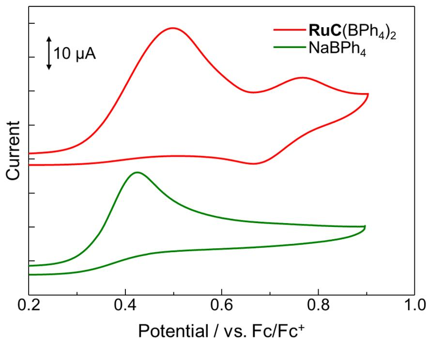
**Fig. S10** CVs of  $\text{RuC}(\text{BPh}_4)_2$  (0.5 mM, red line) and  $\text{NaBPh}_4$  (0.5 mM, green line) in 0.1 M TBAP/MeCN under Ar. Working electrode, glassy carbon; counter electrode, Pt wire; reference electrode, Ag/Ag<sup>+</sup>; scan rate, 0.1 s<sup>-1</sup>. Potential sweeps were started from the open circuit potential for all measurements.
