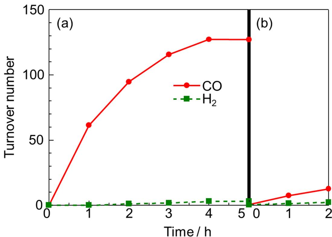
**Fig. S12** (a) Turnover number of the products [CO (red) and H<sub>2</sub> (green)] obtained during the photocatalytic CO<sub>2</sub> reduction (a) with **RuC**(BPh<sub>4</sub>)<sub>2</sub> (20 μM) and BIH (0.10 M) in CO<sub>2</sub>-saturated-MeCN/H<sub>2</sub>O mixture (39:1, v:v) under photoirradiation (420 ≤ λ ≤ 750 nm) at 20 °C, (b) performed using the solution after 5 h reaction in (a) with the addition of BIH (0.10 M).
