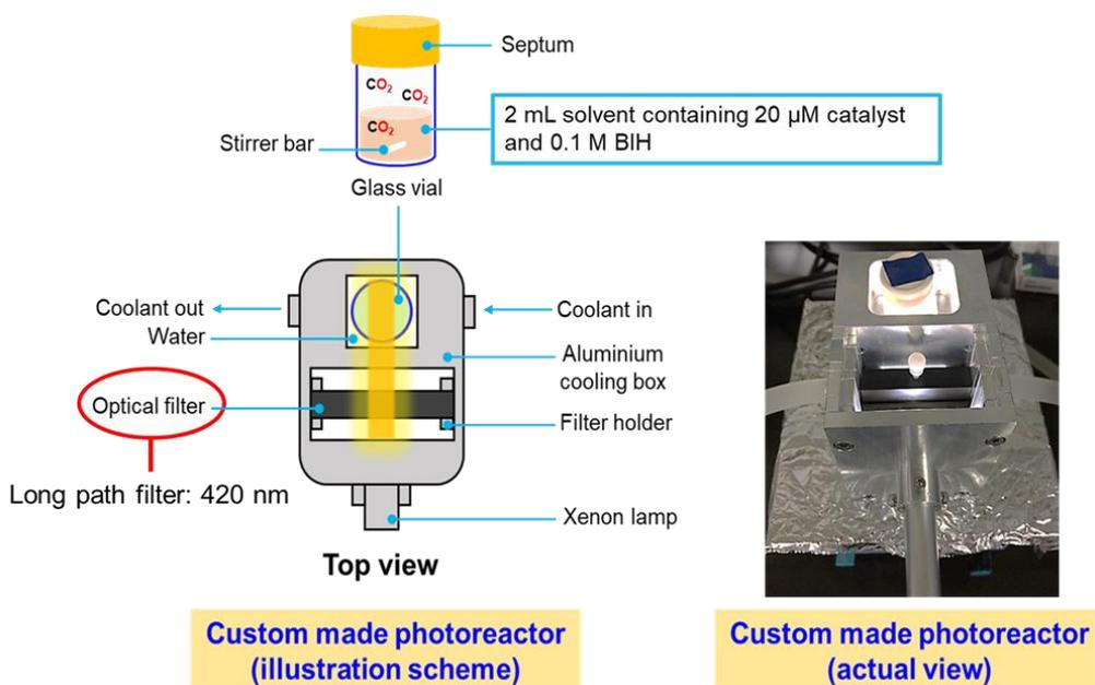
**Fig. S11** Setting of a custom made photoreactor used for photocatalytic CO<sub>2</sub> reduction.
