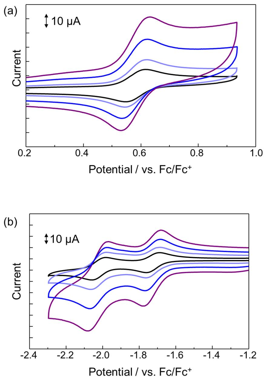
**Fig. S9** CVs of **RuC** (0.5 mM) in 0.1 M TBAP/MeCN under Ar (a) in positive potential region and (b) negative potential region. Working electrode, glassy carbon; counter electrode, Pt wire; reference electrode, Ag/Ag<sup>+</sup>; scan rate, 0.1 s<sup>-1</sup> (black line), 0.2 V s<sup>-1</sup> (pale blue line), 0.5 V s<sup>-1</sup> (blue line) and 1.0 V s<sup>-1</sup> (purple line). Potential sweeps were started from the open circuit potential for all measurements.
