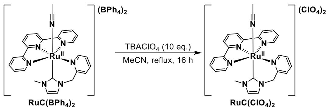
**Scheme S2.** Synthesis of  $\text{RuC}(\text{ClO}_4)_2$ .
