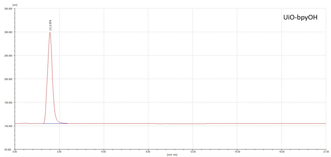
Figure S6. The GC analysis results of UiO-bpyOH and UiO-bpy for EG dehydrogenation at 150°C (the retention time of H 2 is 0.7 min; the peak at 2.3 min is from N 2 )
