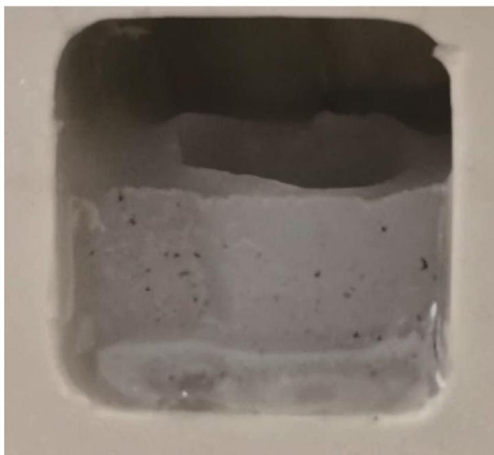
Fig. S19 The optical photograph of 8 mol kg<sup>-1</sup> LiTFSI/H<sub>2</sub>O electrolyte after LSV test at -40 °C.
