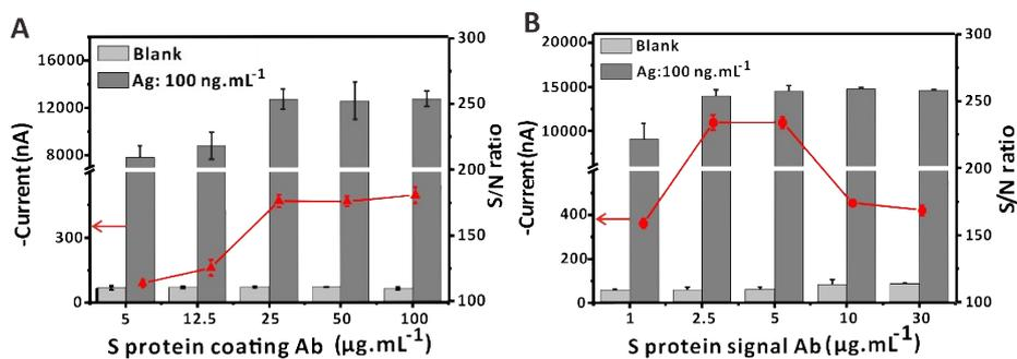
**Figure. S4.** (A) The current value and S/N at the different concentrations of S protein coating antibody, including 5, 12.5, 25, 50 and 100  $\mu\text{g. mL}^{-1}$ , the concentration of S protein: 100  $\text{ng. mL}^{-1}$ . (B) The current value and S/N at the different concentrations of anti-S protein signal antibody, including 1, 2.5, 5, 10 and 30  $\mu\text{g. mL}^{-1}$ , the concentration of S protein antigen: 100  $\text{ng. mL}^{-1}$ .
