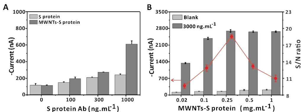
**Figure. S6.** (A) The current value of the electrode modified MWNT-Ag layer compared with the electrode modified with Ag layer only. The concentration of S protein antibody: 100  $\text{ng. mL}^{-1}$ , 300  $\text{ng. mL}^{-1}$ , 1000  $\text{ng. mL}^{-1}$ . (B) The current value and S/N ratio at the different concentrations of MWNTs-S protein conjugate: 0.02  $\text{mg. mL}^{-1}$ , 0.1  $\text{mg. mL}^{-1}$ , 0.25  $\text{mg. mL}^{-1}$ , 0.5  $\text{mg. mL}^{-1}$ , 1  $\text{mg. mL}^{-1}$ .
