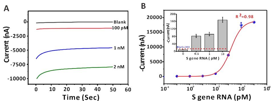
**Figure. S3.** (A) i-t response of 0 and 100 pM, 1 nM, 2 nM of S gene. The potential was held at -0.1 V and the reduction current was recorded at 50 s. (B) The calibration curve of the response current
