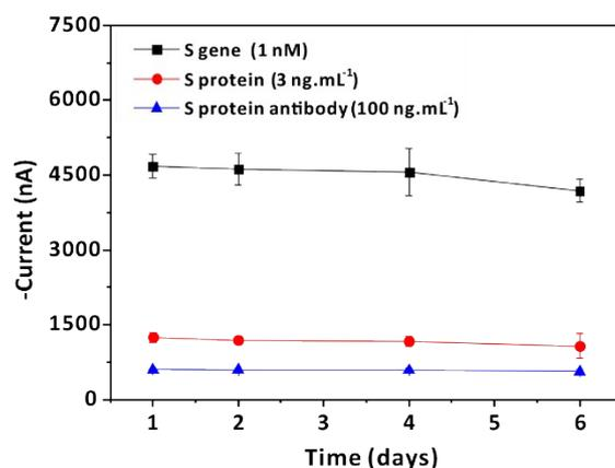
**Figure S8.** The stability study of biosensor against the storage time for 0–6 days. The IT response values of 1nM S gene, 3 ng. mL<sup>-1</sup> S protein and 100 ng. mL<sup>-1</sup>. Standard deviation comes from at least three independent experiments.
