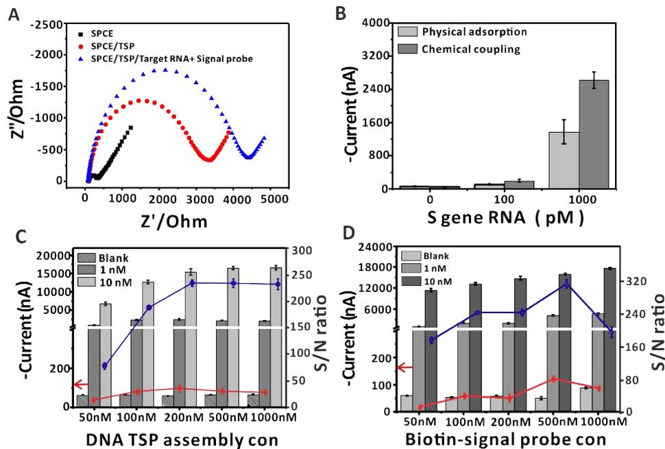
**Figure. S2.** (A) EIS spectra for the assembly of the SARS-CoV-2 S gene of biosensor. The EIS experiments were performed in 0.1 M PBS buffer containing 5 mM  $\text{Fe}(\text{CN})_6^{3-/4-}$ . (B) and (C) Optimization of the amino DNA TSPs assembly method and concentration of DNA TSPs. (D) Optimization of the concentration of biotin-signal probe.
