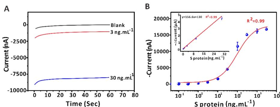
**Figure. S5.** i-t response of the presence of 0, 3  $\text{ng. mL}^{-1}$  and 30  $\text{ng. mL}^{-1}$  target S protein. The potential was held at -0.1 V and the reduction current was recorded at 50 s. (B) The calibration curve of the response current to S protein at a series of concentrations in human serum system, the linear fitting curve of the response current to S protein at low concentration from 0.1  $\text{ng. mL}^{-1}$  to 30  $\text{ng. mL}^{-1}$  (inset D).
