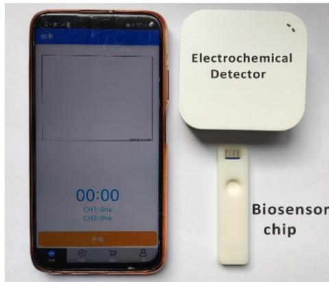
**Figure S1.** A photograph of the smartphone-based electrochemical sensing system
