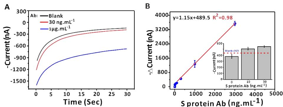
**Figure S7.** (A) *i-t* response of the presence of 0, 30 ng. mL<sup>-1</sup> and 1000 ng. mL<sup>-1</sup> target S protein antibody. The potential was held at -0.1 V and the reduction current was recorded at 30 s. (B) The linear fitting curve of the response current to S protein antibody at a series of concentrations in human serum system (inset D).
