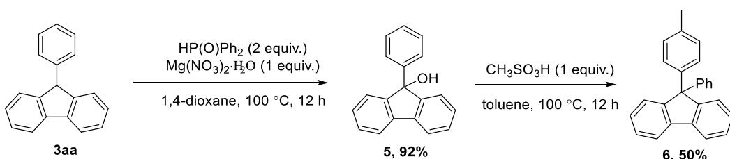
To a solution of **3aa** (60.6 mg, 0.25 mmol) in 1, 4-dioxane (2 mL) was added  $\text{HP(O)Ph}_2$  (101.1 mg,
