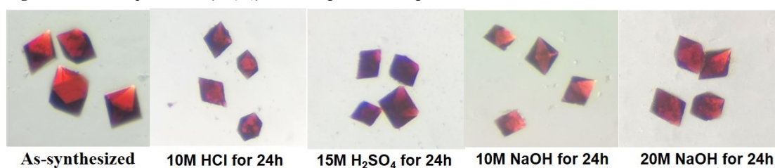
Figure S11. Photographs of fresh crystals and crystal samples after soaking in 15M H_2SO_4 , 12M HCl, 10 M NaOH and 20 M NaOH solutions for 24 hours.
