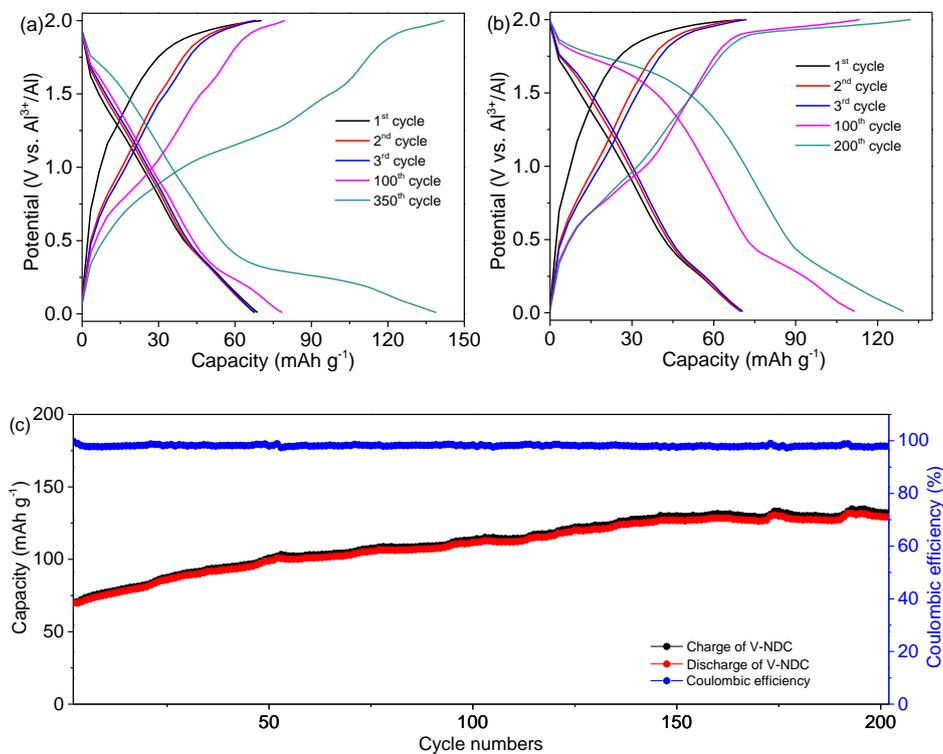
**Fig. S5** (a) Charge-discharge curves of V-NDC at  $0.3 \text{ A g}^{-1}$ . (b) Charge-discharge curves and (c) cycling performance of V-NDC with a loading of  $2.23 \text{ mg cm}^{-2}$  cycling at  $0.2 \text{ A g}^{-1}$ .
