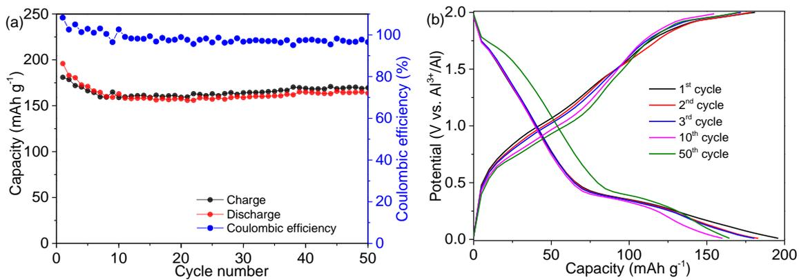
**Fig. S6** (a) Capacity and (b) charge-discharge curves of pure V<sub>2</sub>O<sub>3</sub> at 0.3 A g<sup>-1</sup>.
