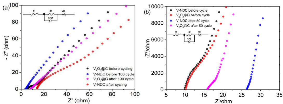
**Fig. S12** EIS spectra of different samples at (a) room temperature and (b)  $-10 \text{ }^\circ\text{C}$ .
