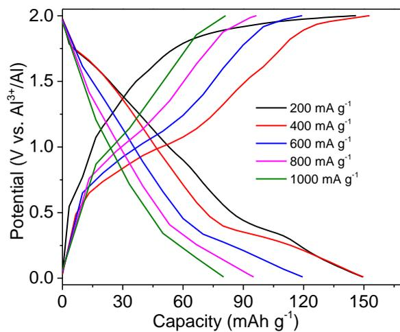
**Fig. S8** Charge-discharge profiles of V<sub>2</sub>O<sub>3</sub>@C during rate-performance measurements.
