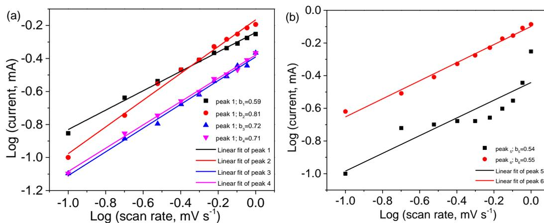
**Fig. S15** The  $\log(i)$  vs.  $\log(v)$  of (a) oxidization and (b) reduction peaks.
