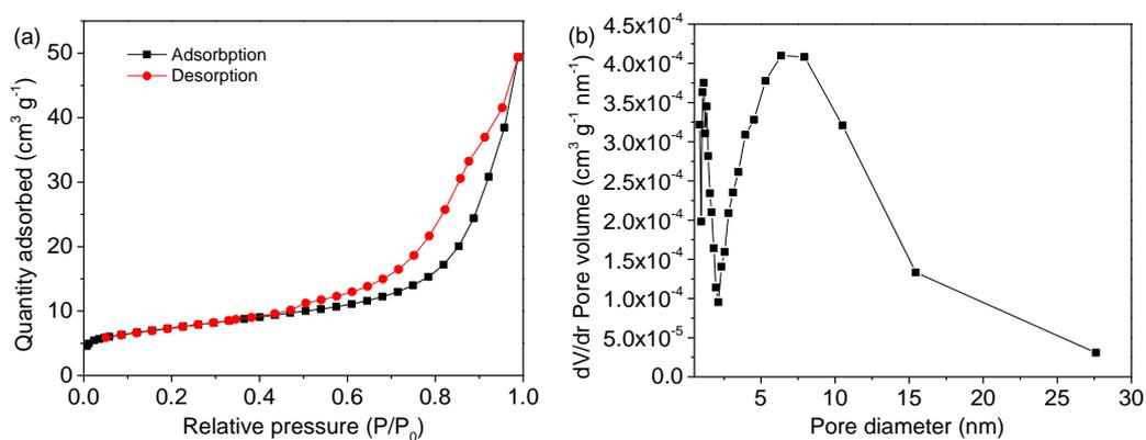
**Fig. S3** (a) Adsorption-desorption isotherm and (b) pore-size distribution of  $V_2O_5@C$ .
