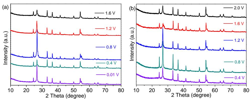
**Fig. S10** *Ex-situ* XRD patterns of V<sub>2</sub>O<sub>3</sub>@C composite at different potentials during (a) discharge and (b) charge.
