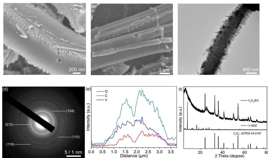
**Fig. S1** (a) SEM image of the book-like lamellar  $\text{V}_2\text{O}_3@\text{C}$  calcined at 600  $^\circ\text{C}$ ; (b) SEM image, (c) TEM image, (d) SAED pattern, and (e) line-scanning curves of  $\text{V}_2\text{O}_3@\text{C}$  calcined at 800  $^\circ\text{C}$ . (f) XRD patterns of V-NDC and  $\text{V}_2\text{O}_3@\text{C}$ .
