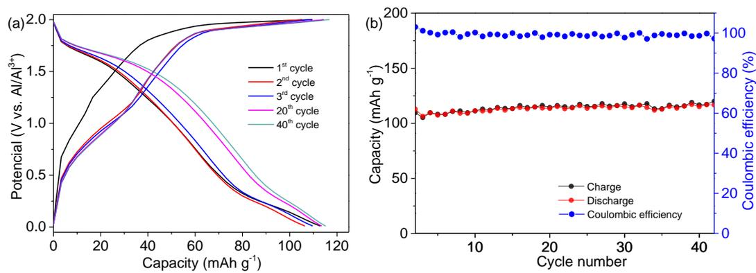
**Fig. S9** (a) Charge-discharge profiles and (b) cycling performance of V-NDC at  $-10\text{ }^{\circ}\text{C}$ .
