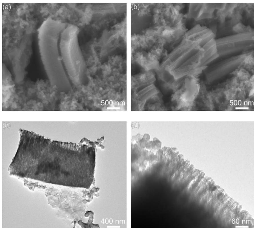
**Fig. S13** (a,b) SEM images, (c,d) TEM images of  $V_2O_3@C$  after 50 cycles at  $0.3 \text{ A g}^{-1}$  at  $-10 \text{ }^\circ\text{C}$ .
