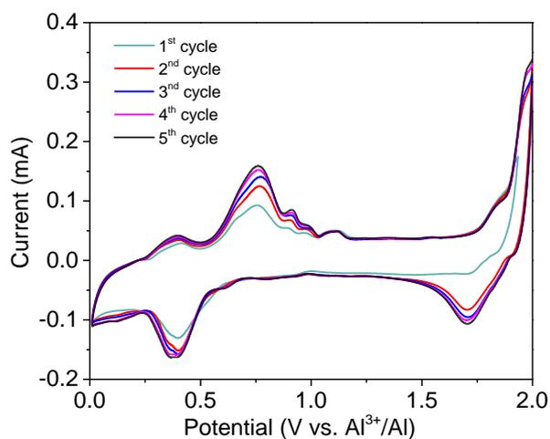
**Fig. S7** CV profiles of V-NDC at a scanning rate of 0.1 mV s<sup>-1</sup>.
