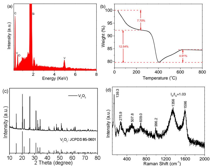
**Fig. S2** (a) EDS spectrum and (b) TGA curve of  $V_2O_5@C$ . (c) XRD pattern of the sample after TGA measurement. (d) Raman spectrum of  $V_2O_5@C$ .
