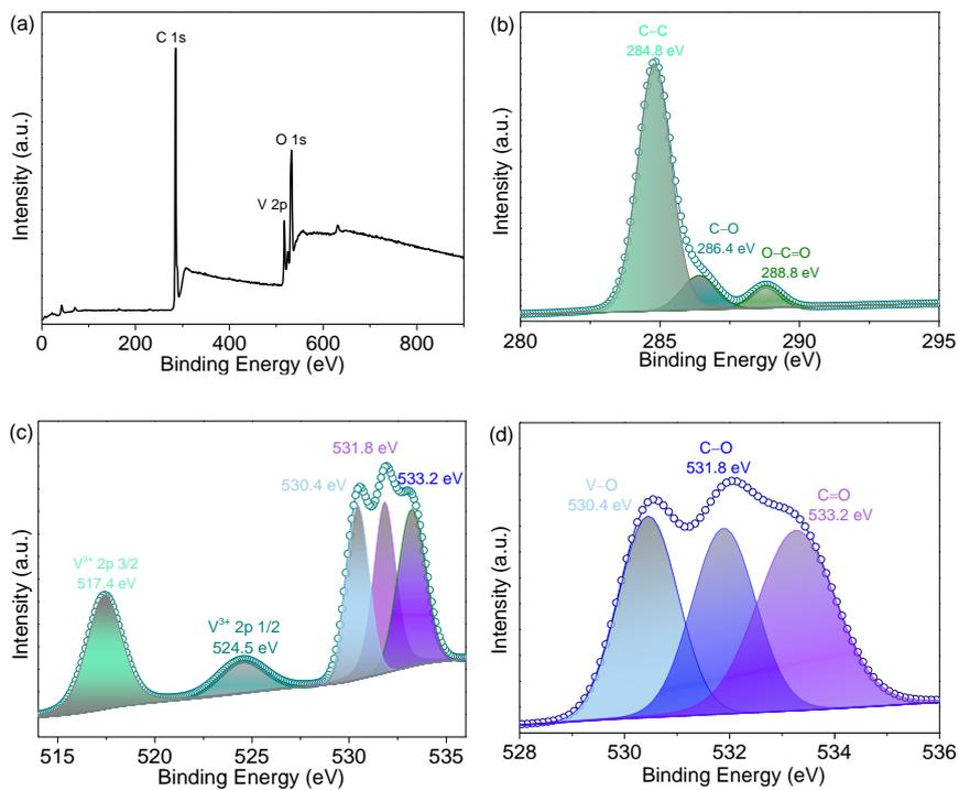
**Fig. S4** XPS spectra of  $V_2O_3@C$ : (a) full survey spectrum, (b) C 1s, (c) V 2p, and (d) O 1s.
