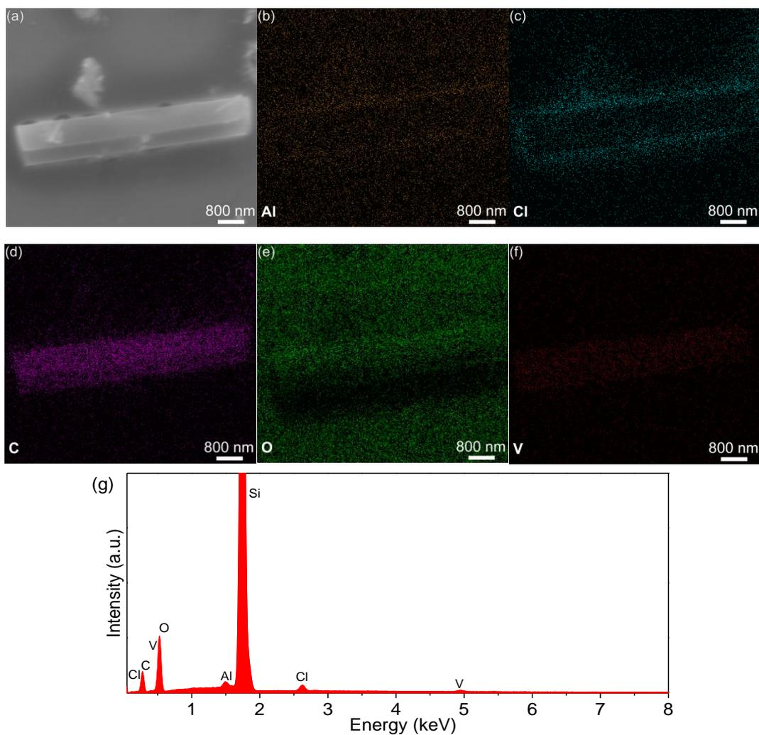
**Fig. S11** (a) SEM image, (b-f) Al, Cl, C, O, V elemental mapping images and (g) EDS spectrum of  $V_2O_3@C$  after 50 cycles at  $0.3 \text{ A g}^{-1}$ .
