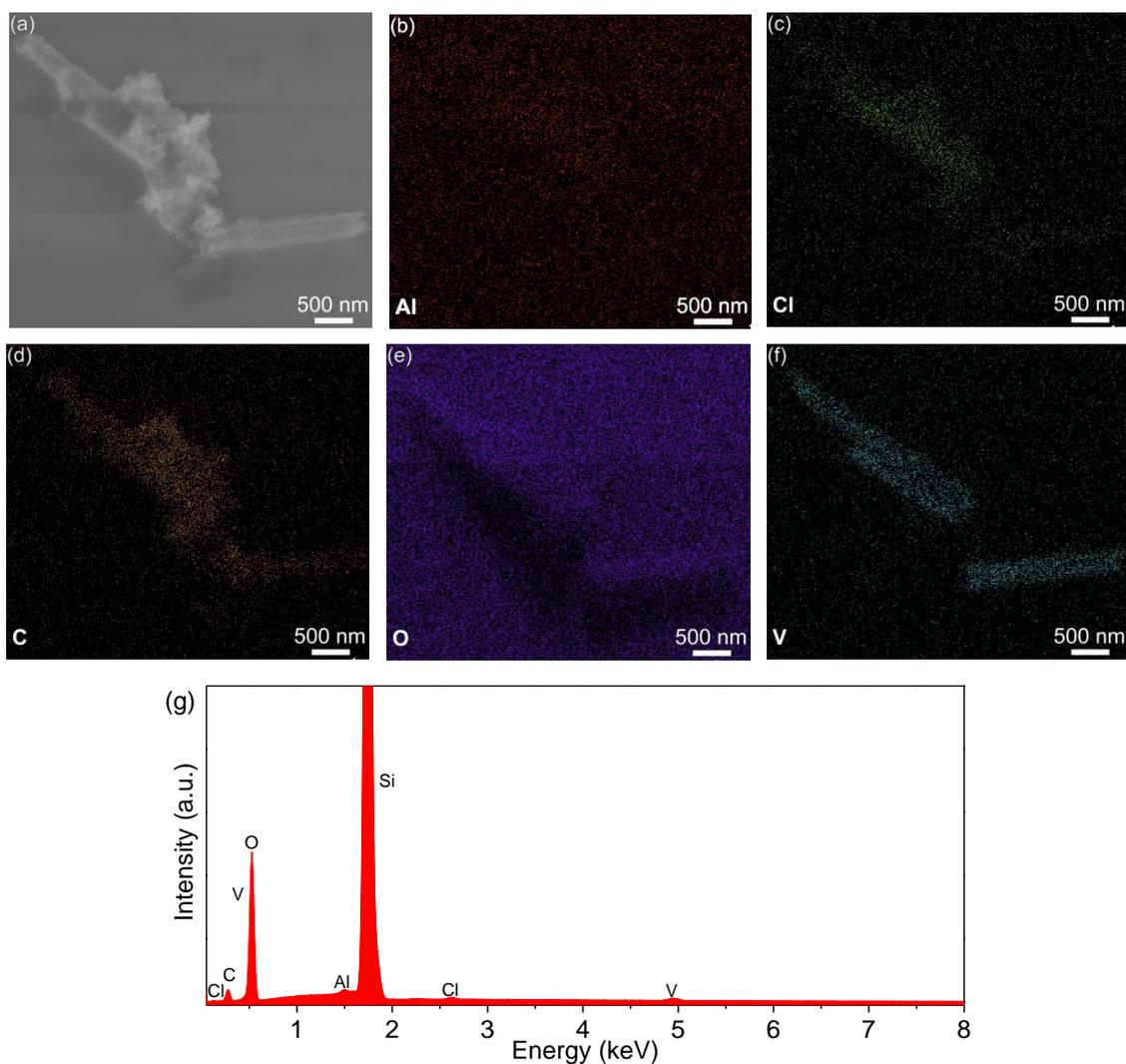
**Fig. S14** (a) SEM images, (b-f) elemental mapping and (g) EDS spectrum of  $V_2O_3@C$  after 50 cycles at  $0.3 \text{ A g}^{-1}$  at  $-10 \text{ }^\circ\text{C}$ .
