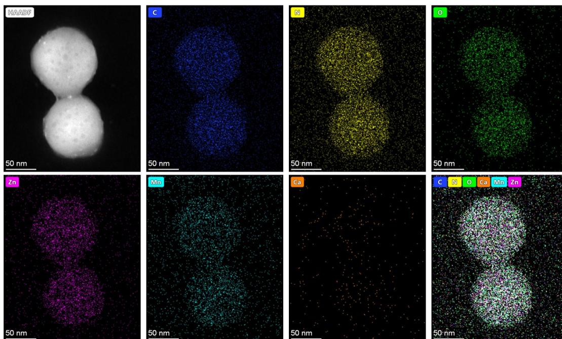
**Figure S2.** STEM elementary distribution of the MnCaCZ: The high-angle annular dark-field image (HAADF) of the NPs; elements distribution of C, N, O, Zn, Mn and Ca; The overlap of all elements.
