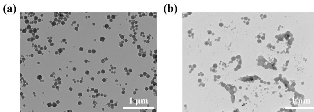
**Figure S4.** TEM images of the MnCaCZ NPs after immersion in PBS at pH = (a) 7.4 and (b) 5.0.
