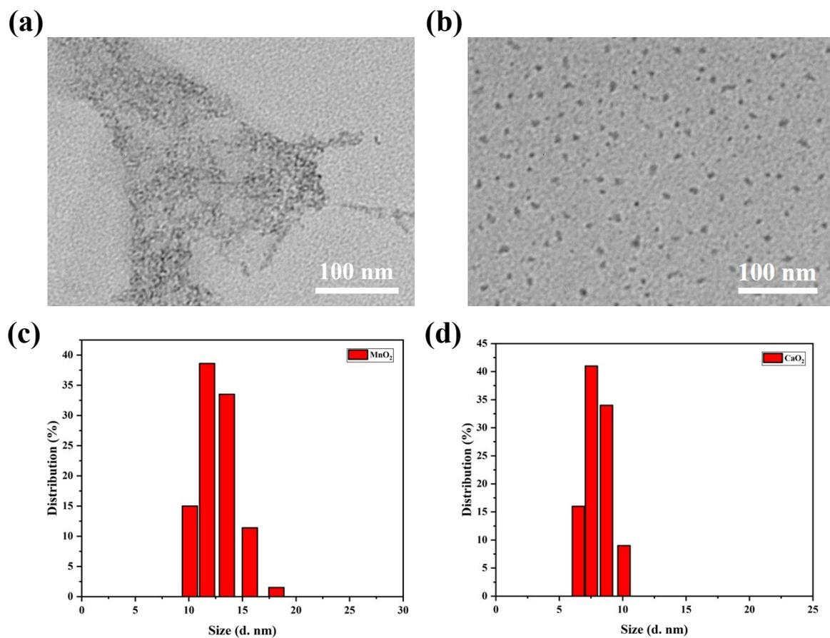
**Figure S1.** TEM image of (a) the MnO<sub>2</sub> NPs and (b) the CaO<sub>2</sub> NPs; DLS results of (c) the MnO<sub>2</sub> NPs and (d) the CaO<sub>2</sub> NPs.
