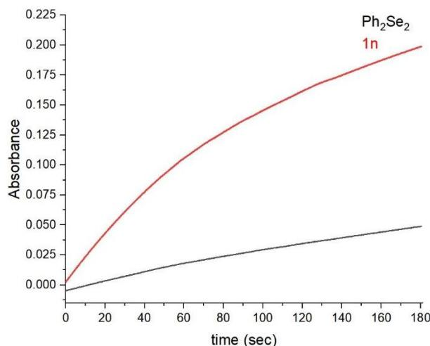
**Figure S1.** A model plot of absorbance *vs* time (sec). The initial concentration of benzenethiol, catalyst **1n** (0.1 mM) and H<sub>2</sub>O<sub>2</sub> were fixed to 3.75 mM.
