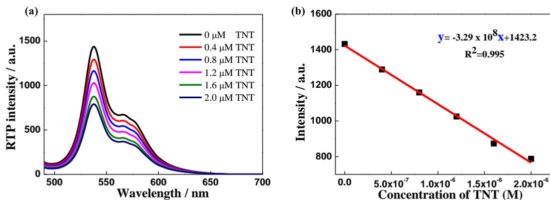
**Figure S43.** Emission spectra of 10  $\mu\text{M}$  Au- $\gamma$ -Rot in the presence of lower concentration of TNT (a) in aerated  $\text{H}_2\text{O}$  at 25  $^\circ\text{C}$ .  $\lambda_{\text{ex}}=330$  nm in phosphorescence mode, and its corresponding detection limit plot (b). TNT was dissolved in DMF mother solution.
