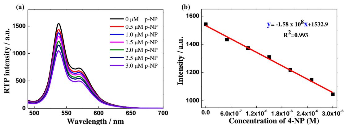
**Figure S46.** Emission spectra of 10  $\mu\text{M}$  **Au- $\gamma$ -Rot** in the presence of lower concentration of **p-NP** (a) in aerated  $\text{H}_2\text{O}$  at 25  $^\circ\text{C}$ .  $\lambda_{\text{ex}}=330$  nm in phosphorescence mode, and its corresponding detection limit plot (b). **p-NP** was dissolved in DMF mother solution.
