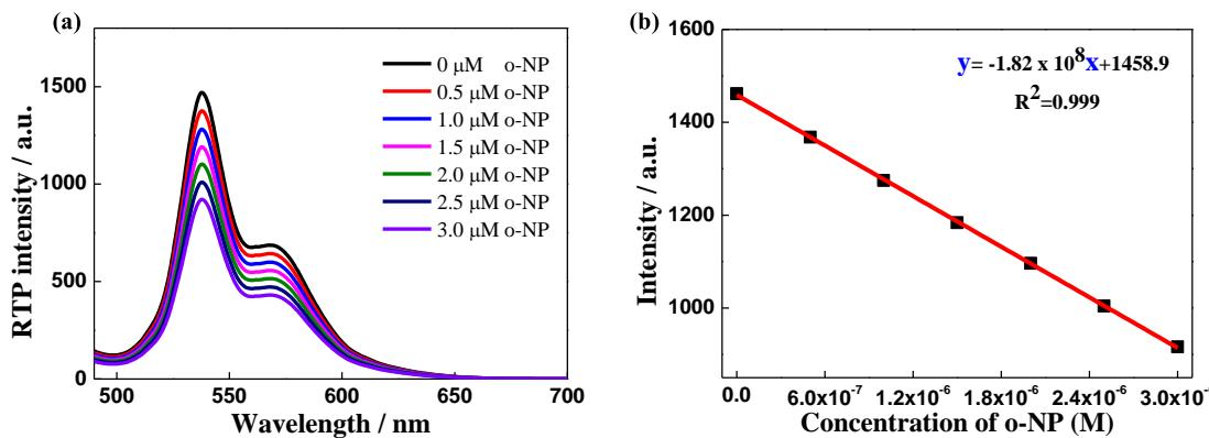
**Figure S44.** Emission spectra of  $10 \mu\text{M}$  **Au- $\gamma$ -Rot** in the presence of lower concentration of **o-NP** (a) in aerated  $\text{H}_2\text{O}$  at  $25^\circ\text{C}$ .  $\lambda_{\text{ex}}=330 \text{ nm}$  in phosphorescence mode, and its corresponding detection limit plot (b). **o-NP** was dissolved in DMF mother solution.
