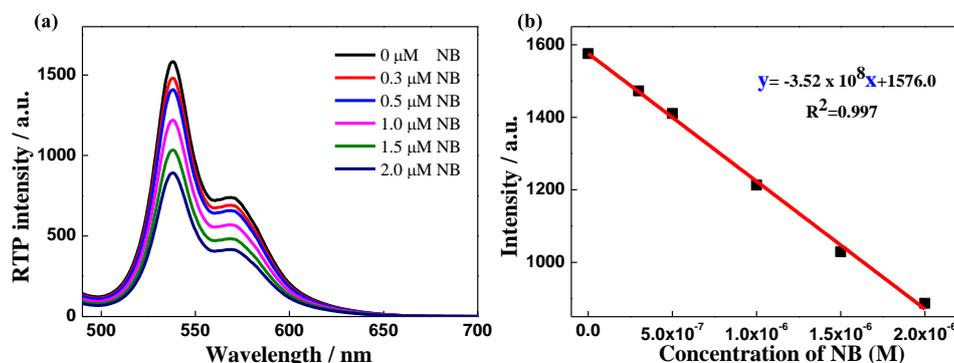
**Figure 42.** Emission spectra of 10 μM **Au-γ-Rot** in the presence of lower concentration of **NB** (a) in aerated H<sub>2</sub>O at 25 °C.  $\lambda_{\text{ex}}=330$  nm in phosphorescence mode, and its corresponding detection limit plot (b). **NB** was dissolved in DMF mother solution.
