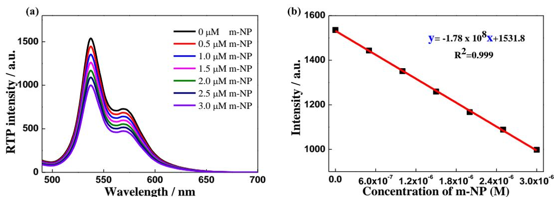
**Figure S45.** Emission spectra of 10  $\mu\text{M}$  Au- $\gamma$ -Rot in the presence of lower concentration of m-NP (a) in aerated  $\text{H}_2\text{O}$  at 25  $^\circ\text{C}$ .  $\lambda_{\text{ex}}=330$  nm in phosphorescence mode, and its corresponding detection limit plot (b). m-NP was dissolved in DMF mother solution.
