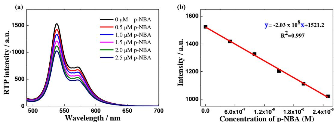
**Figure S47.** Emission spectra of 10  $\mu\text{M}$  **Au- $\gamma$ -Rot** in the presence of lower concentration of **p-NBA** (a) in aerated  $\text{H}_2\text{O}$  at 25  $^\circ\text{C}$ .  $\lambda_{\text{ex}}=330$  nm in phosphorescence mode, and its corresponding detection limit plot (b). **p-NBA** was dissolved in DMF mother solution.
