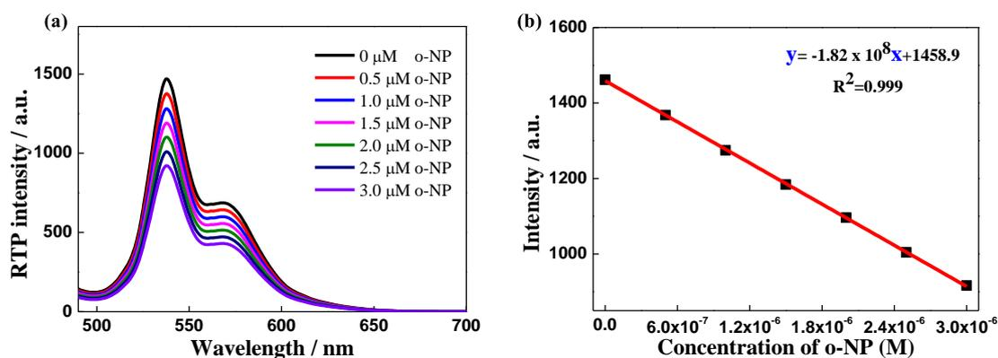
**Figure S44.** Emission spectra of 10  $\mu\text{M}$  Au- $\gamma$ -Rot in the presence of lower concentration of o-NP (a) in aerated  $\text{H}_2\text{O}$  at 25  $^\circ\text{C}$ .  $\lambda_{\text{ex}}=330$  nm in phosphorescence mode, and its corresponding detection limit plot (b). o-NP was dissolved in DMF mother solution.
