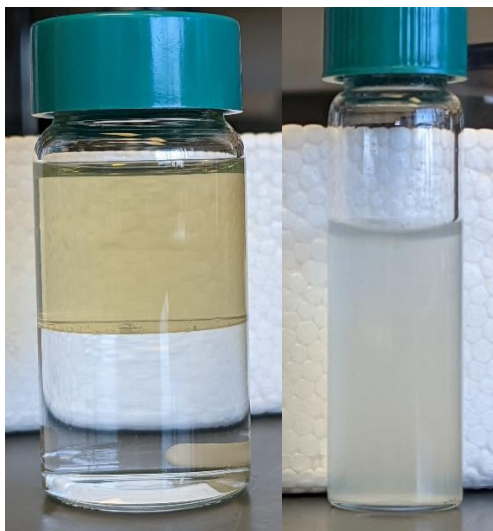
Figure S1. CIO NCs at the beginning of base stripping (left) and after stripping and purification (right).
