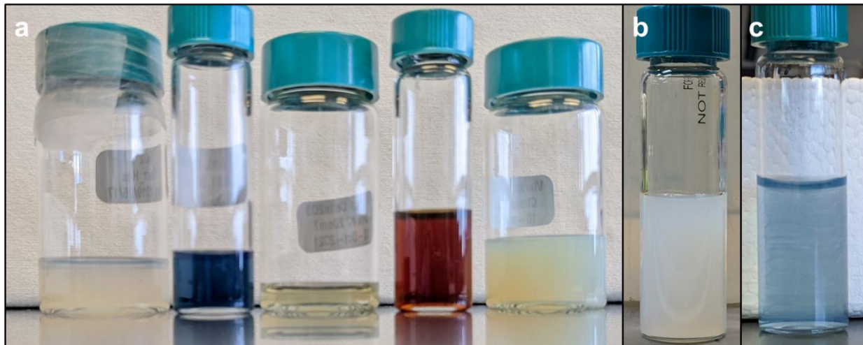
Figure S6. a) Ligand capped dispersions of (left to right), \text{TiO}_2 , ITO, CIO, \text{CeO}_2 , UIO. Aqueous ligand stripped dispersions of b) \text{TiO}_2 and c) ITO.
