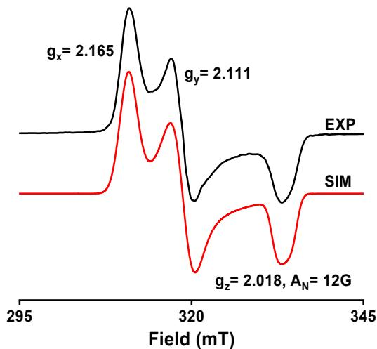
**Figure S14.** Experimental (THF:2MeTHF (1:3) glass, 77 K) and simulated EPR spectra of  $[(Me_3TACN)Ni^I(CN^tBu)_2]^+$ . The following parameters were used for simulations:  $g_x = 2.165$ ;  $g_y = 2.111$ ;  $g_z = 2.018$  ( $A_N = 12.0$  G).
