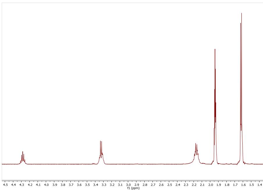
**Figure S1.** <sup>1</sup>H NMR for [(iPr<sub>3</sub>TACN)Ni<sup>II</sup>NO]PF<sub>6</sub>, **2**, (500 MHz, CD<sub>3</sub>CN)  $\delta$  4.29 (hept,  $J = 6.5$  Hz, 3H), 3.38 – 3.26 (m, 6H), 2.25 – 2.10 (m, 6H), 1.62 (d,  $J = 6.7$  Hz, 18H).
