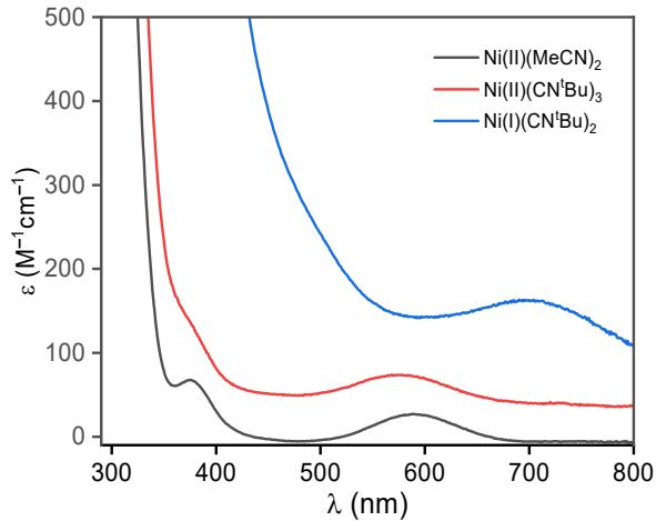
**Figure S12.** Overlayed UV-vis absorption spectra for  $[(iPr_3TACN)Ni^{II}(MeCN)_3](PF_6)_2$  (black),  $[(iPr_3TACN)Ni^{II}(CN^tBu)_3](PF_6)_2$  (red), and  $[(iPr_3TACN)Ni^I(CN^tBu)_2](PF_6)$  (blue) in MeCN.
