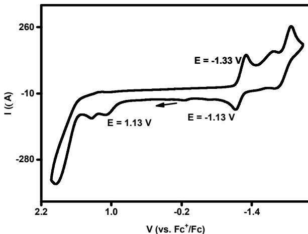
**Figure S7.** CV of  $[(\text{iPr}_3\text{TACN})\text{Ni}^{\text{II}}(\text{MeCN})_2](\text{PF}_6)_2$  in 0.1 M  $n\text{-Bu}_4\text{NPF}_6/\text{MeCN}$  (100 mV/s scan rate). The  $\text{Ni}^{\text{II}}/\text{Ni}^{\text{I}}$  reduction potential was observed at  $E_{1/2} = -1.23 \text{ V}$ .
