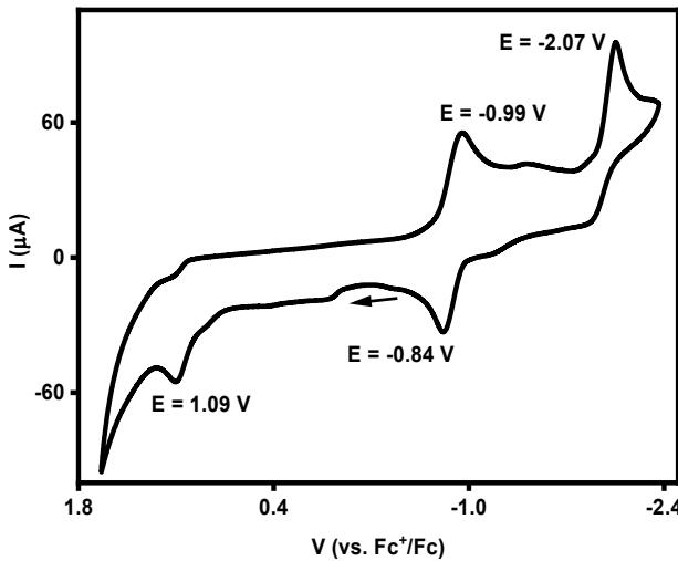
**Figure S8.** CV of  $[(\text{iPr}_3\text{TACN})\text{Ni}^{\text{II}}(\text{CN}^t\text{Bu})_3](\text{PF}_6)_2$  in 0.1 M  $n\text{-Bu}_4\text{NPF}_6/\text{MeCN}$  (100 mV/s scan rate). The  $\text{Ni}^{\text{II}}/\text{Ni}^{\text{I}}$  reduction potential was observed at  $E_{1/2} = -0.92 \text{ V}$ .
