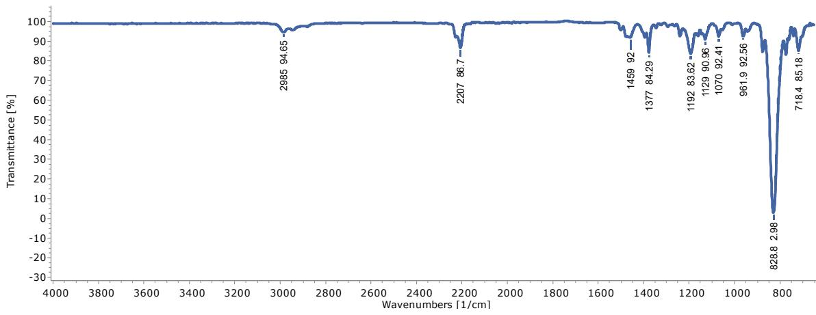
**Figure S5.** IR spectrum of  $[(iPr_3TACN)Ni^{II}(CN^tBu)_3](PF_6)$  from bulk THF reaction. IR ( $\text{cm}^{-1}$ ): 718 (m), 829 (s), 962 (m), 1070 (m), 1129 (m), 1192 (m), 1377 (m), 1459 (m), 2207 (m), 2232 (sh), 2985 (m).
