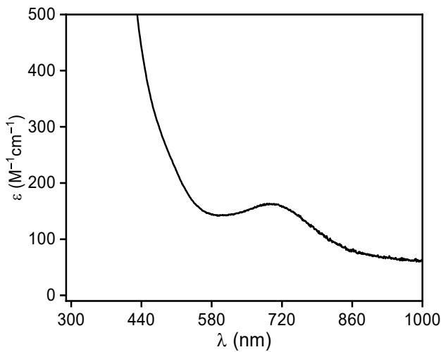
**Figure S11.** UV-vis absorption spectrum of  $[(iPr_3TACN)Ni^I(CN^tBu)_2](PF_6)$  (1.6 mM in MeCN).
