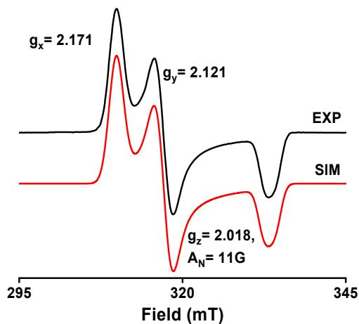
**Figure S13.** Experimental (MeCN:PrCN (1:3) glass, 77 K) and simulated EPR spectra of  $[(iPr_3TACN)Ni^I(CN^tBu)_2]^+$  (**5**) The following parameters were used for simulations:  $g_x = 2.171$ ;  $g_y = 2.121$ ;  $g_z = 2.018$  ( $A_N = 11.0$  G).
