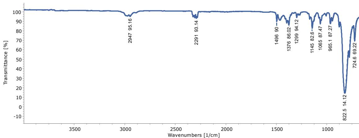
**Figure S4.** IR spectrum of  $[(iPr_3TACN)Ni^{II}(MeCN)_2](PF_6)_2$ . IR ( $\text{cm}^{-1}$ ): 383 (m), 557 (s), 723 (m), 832 (s), 965 (m), 1065 (m), 1155 (m), 1299 (m), 1375 (m), 1496 (m), 2291 (m), 2947 (m).
