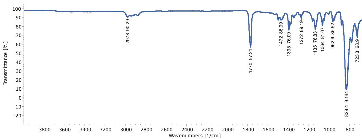
**Figure S3.** IR spectrum of  $[(iPr_3TACN)Ni^{II}NO]PF_6$ . IR ( $\text{cm}^{-1}$ ): 723 (m), 829 (s), 962 (m), 1064 (m), 1135 (m), 1272 (m), 1395 (m), 1472 (m), 1770 (m), 2978 (m)
