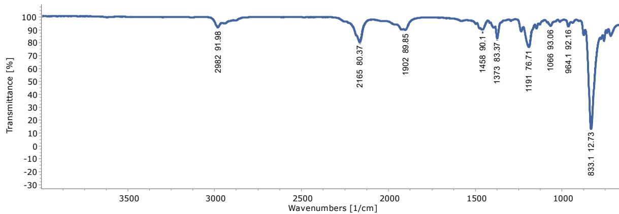
**Figure S6.** IR spectrum of  $[(iPr_3TACN)Ni^I(CN^tBu)_2](PF_6)$ . IR ( $\text{cm}^{-1}$ ): 833 (s), 964 (m), 1066 (m), 1192 (m), 1373 (m), 1458 (m), 1902 (m), 2165 (m), 2185 (sh), 2982 (m).
