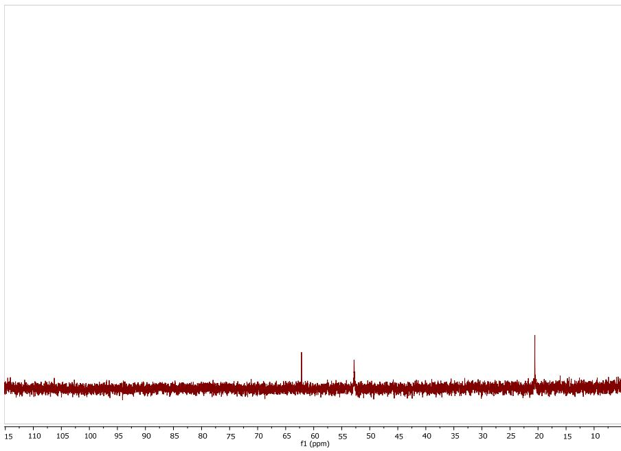
**Figure S2.** <sup>13</sup>C NMR for [(iPr<sub>3</sub>TACN)Ni<sup>II</sup>NO]PF<sub>6</sub>, **2**, (500 MHz, CD<sub>3</sub>CN)  $\delta$  20.57, 52.80, 62.17
