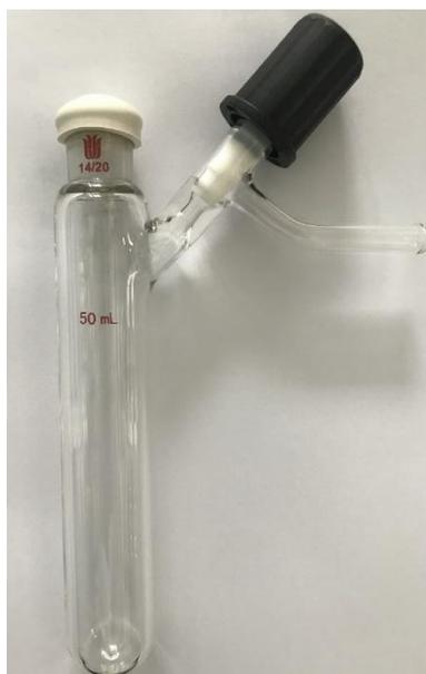
Fig. S23 The photograph of photocatalytic reactor.
