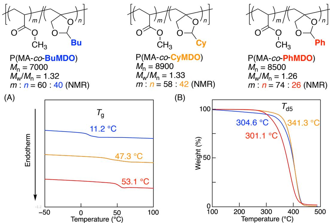
**Figure S18.** Differential scanning calorimetry (DSC) curves (A) and thermogravimetric analysis (TGA) curves (B) of the copolymers obtained in the RAFT copolymerization of cyclic vinyl ethers with MA.
