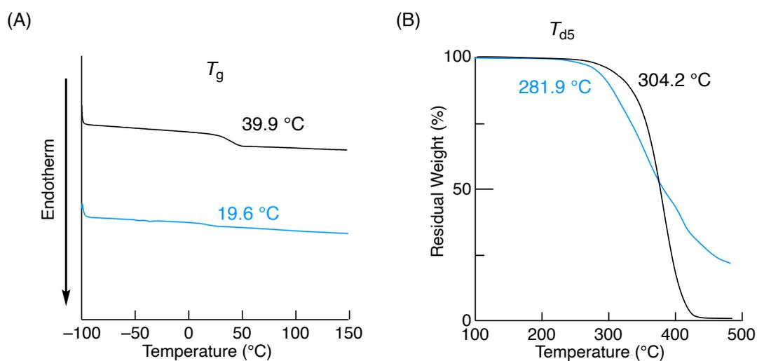
**Figure S23.** DSC curves (A) and TGA curves (B) of PMA-*b*-P(MA-*co*-PhMDO) (black lines) and the copolymer obtained after acetal deprotection (blue lines).
