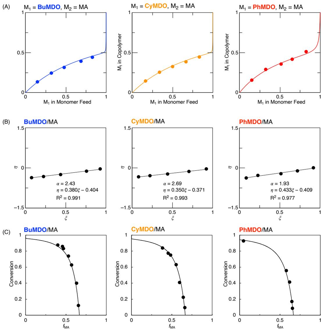
**Figure S17.** Copolymer composition curves for the radical copolymerization (A), Kelen–Tüdös plots (B) and Meyer-Lowry plots<sup>2</sup> (C) for determining monomer reactivity ratio of cyclic vinyl ethers as M<sub>1</sub> and MA as M<sub>2</sub>.
