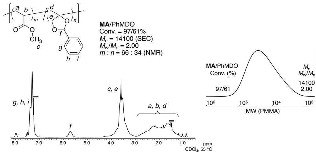
**Figure S9.**  $^1H$  NMR spectrum and SEC curve of random copolymer obtained from the radical copolymerization of PhMDO and MA.
