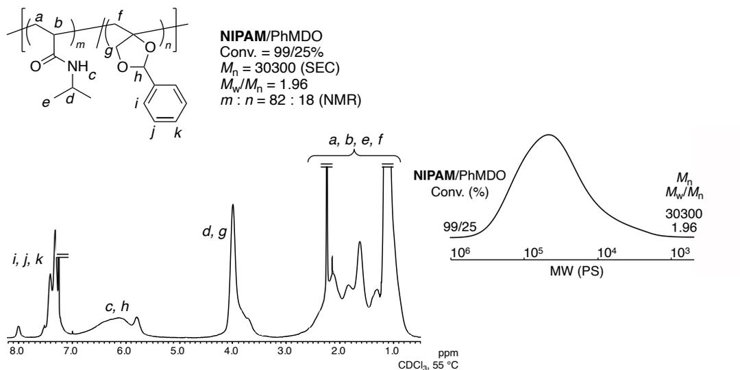
**Figure S13.**  $^1H$  NMR spectrum and SEC curve of random copolymer obtained from the radical copolymerization of PhMDO and NIPAM.
