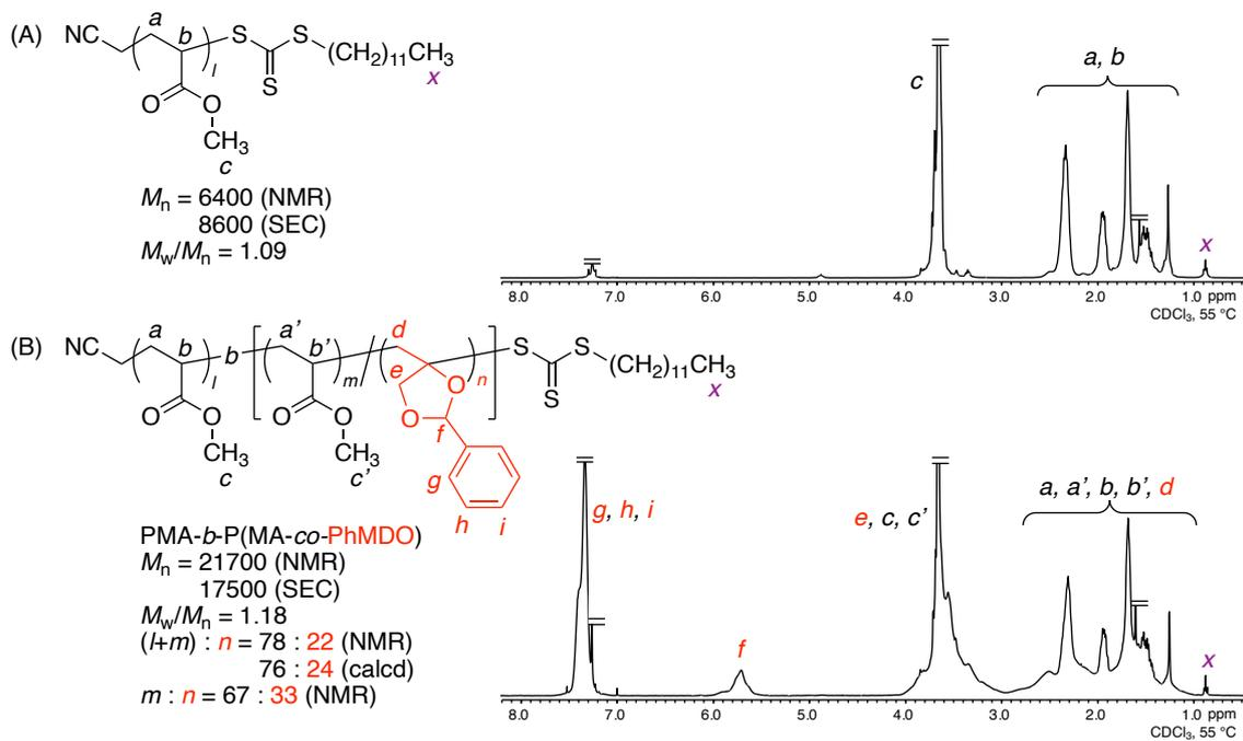
**Figure S19.**  $^1\text{H}$  NMR spectra of PMA (A) and the continuing PMA-*b*-P(MA-*co*-PhMDO) (B) obtained from the RAFT block copolymerization of vinyl ethers and MA.  $[\text{MA}]_0/[\text{CMDTTC}]_0/[\text{V-70}]_0 = 3750/25/6.25$  mM;  $[\text{PhMDO}]_{\text{add}} = 1500$  mM in toluene at  $20^\circ\text{C}$ .
