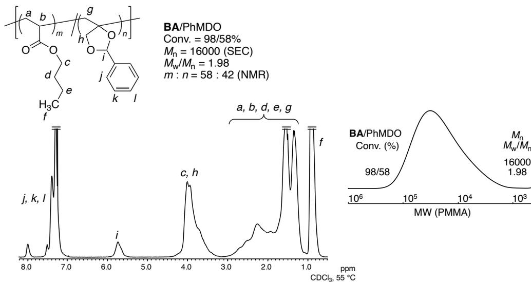
**Figure S10.**  $^1H$  NMR spectrum and SEC curve of random copolymer obtained from the radical copolymerization of PhMDO and BA.
