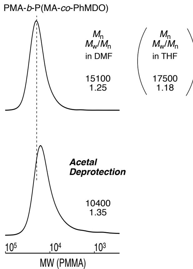
**Figure S21.** SEC curves (in DMF containing LiBr as the eluent) of block copolymer PMA-*b*-P(MA-*co*-PhMDO) (A) before and (B) after acetal deprotection.
