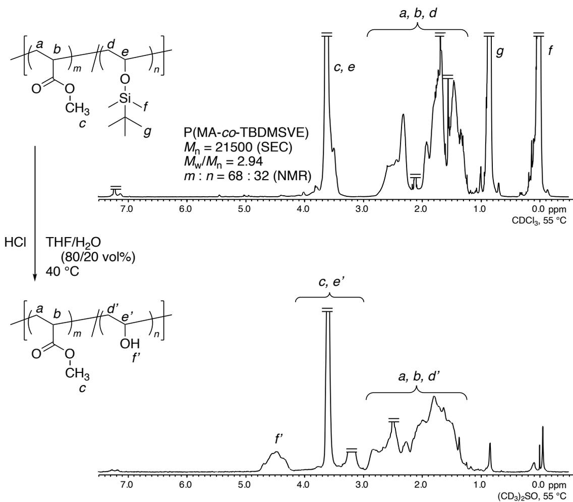
**Figure S22.** <sup>1</sup>H NMR spectra of random copolymer P(MA-co-TBDMSVE) before and after silyl deprotection (98% deprotection).
