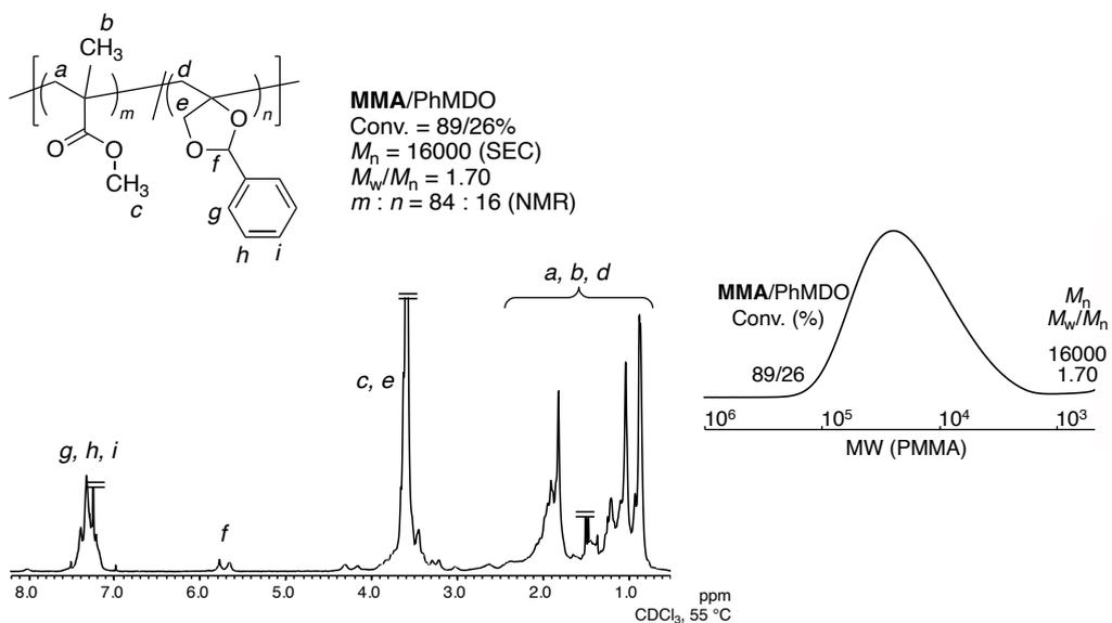
**Figure S12.** <sup>1</sup>H NMR spectrum and SEC curve of random copolymer obtained from the radical copolymerization of PhMDO and MMA.
