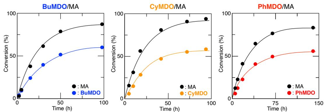
**Figure S14.** Time-conversion for the RAFT copolymerization of glycerol-derived cyclic vinyl ethers and MA:  $[VE]_0/[MA]_0/[CPBD]_0/[AIBN]_0 = 1500/1500/20/5.0$  mM in toluene at  $60^\circ C$ .
