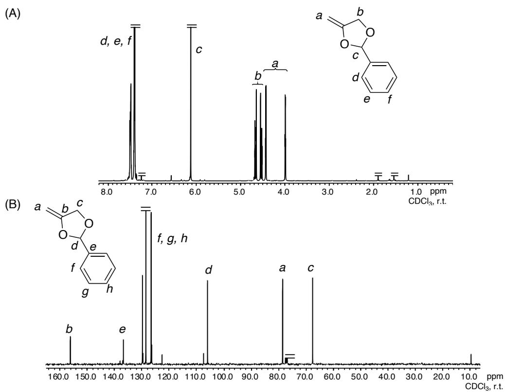
**Figure S8.**  $^1\text{H}$  NMR (A) and  $^{13}\text{C}$  NMR (B) spectra of 4-methylene-2-phenyl-1,3-dioxolane (PhMDO).
