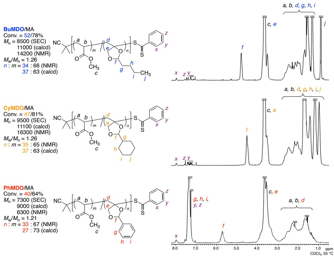
**Figure S16.**  $^1\text{H}$  NMR spectra of random copolymers obtained from the RAFT copolymerization of vinyl ethers and MA:  $[\text{VE}]_0/[\text{MA}]_0/[\text{CPBD}]_0/[\text{AIBN}]_0 = 1500/1500/20/5.0$  mM in toluene at  $60^\circ\text{C}$ .
