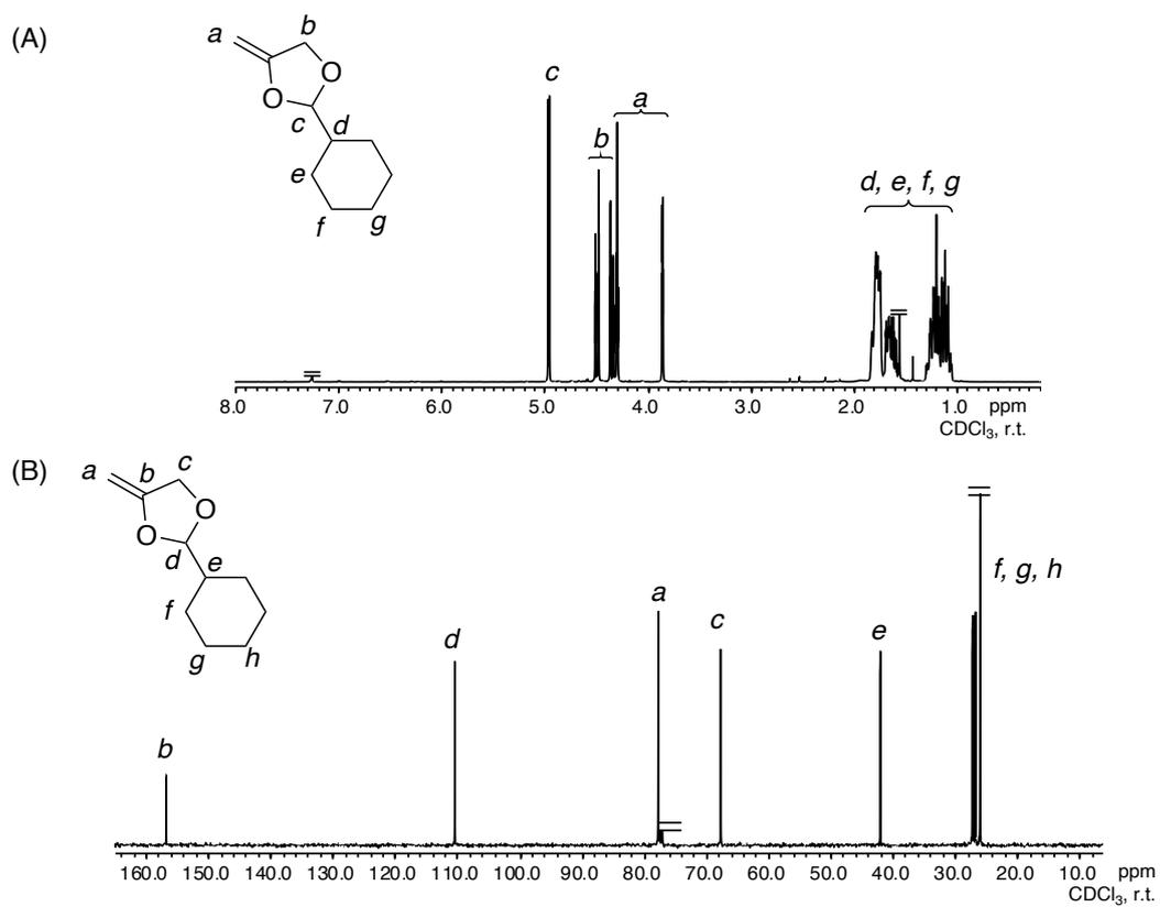
**Figure S6.**  $^1\text{H}$  NMR (A) and  $^{13}\text{C}$  NMR (B) spectra of 2-cyclohexyl-4-methylene-1,3-dioxolane (CyMDO).
