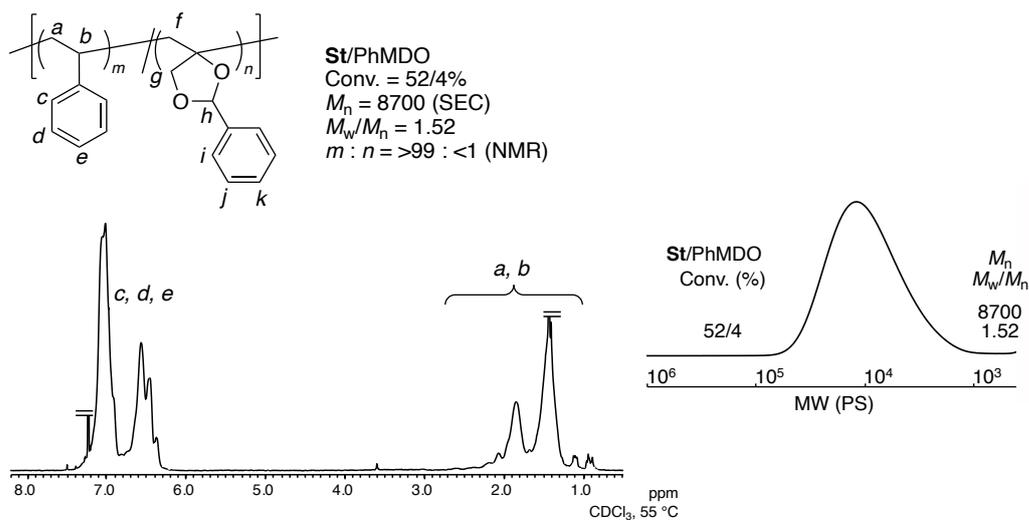
**Figure S11.** <sup>1</sup>H NMR spectrum and SEC curve of random copolymer obtained from the radical copolymerization of PhMDO and St.
