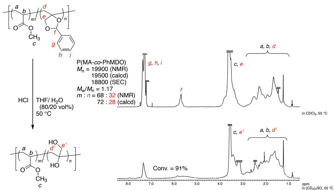
**Figure S20.** <sup>1</sup>H NMR spectra of random copolymer P(MA-co-PhMDO) before and after acetal deprotection.
