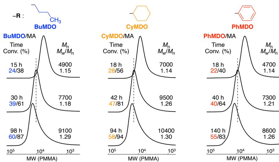
**Figure S15.** SEC curves for the RAFT copolymerization of glycerol-derived cyclic vinyl ethers and MA:  $[\text{VE}]_0/[\text{MA}]_0/[\text{CPBD}]_0/[\text{AIBN}]_0 = 1500/1500/20/5.0$  mM in toluene at 60 °C.
