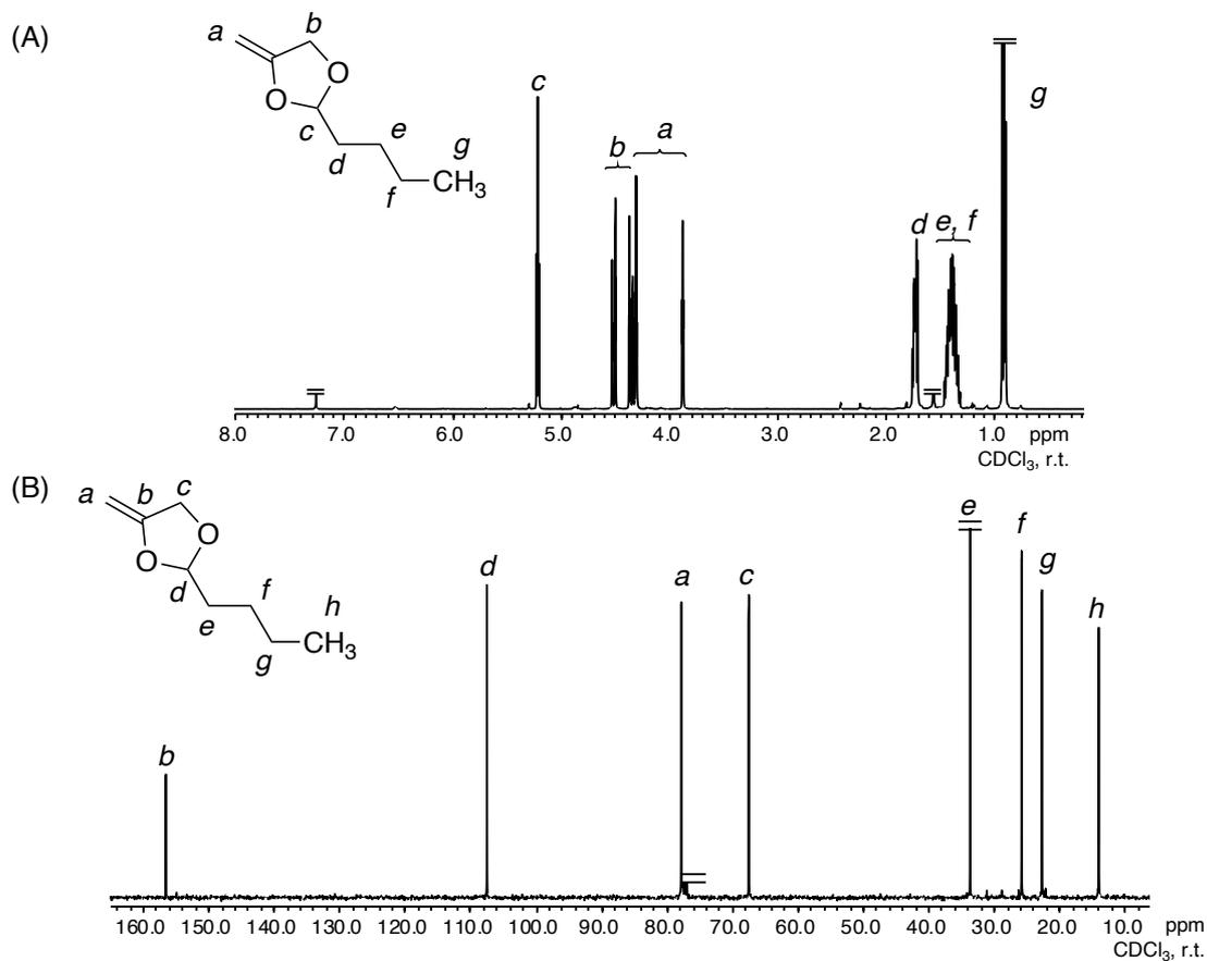
**Figure S4.**  $^1\text{H}$  NMR (A) and  $^{13}\text{C}$  NMR (B) spectra of 2-butyl-4-methylene-1,3-dioxolane (BuMDO).
