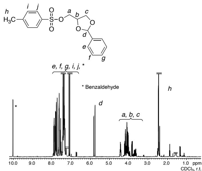
**Figure S7.**  $^1\text{H}$  NMR spectrum of 2-phenyl-4-tosyloxymethyl-1,3-dioxolane.
