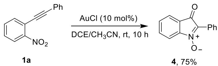
Under N<sub>2</sub> atmosphere, a 10 mL oven-dried flask was charged with AuCl (10 mol%, 4.64 mg), *o*-nitroalkynes **1** (0.2 mmol, 44.6 mg) with anhydrous DCE (1.0 mL) and anhydrous CH<sub>3</sub>CN (1.0 mL). Then the reaction vessel was stirred at rt for 10 h. After the reaction is completed, the solution was purified by flash column chromatography on silica gel (petroleum ether/ethyl acetate = 50:1) to give a red solid **4** in 75% yield (**4** was detected by <sup>1</sup>H NMR and HRMS).
