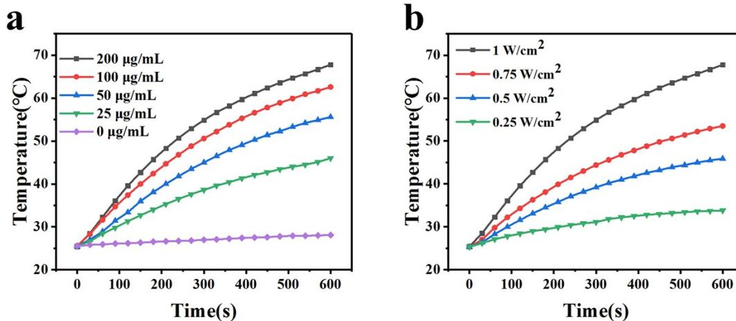
**Figure S16.** (a) Photothermal heating curves of FeSA-HNCSB nanozyme under a NIR laser (808 nm, 1.0 W cm<sup>-2</sup>) at different concentrations for 600 s and (b) photothermal heating curves of FeSA-HNCSB nanozyme (200 µg mL<sup>-1</sup>, 1 mL) with different power density of 808 nm laser irradiation for 600 s.
