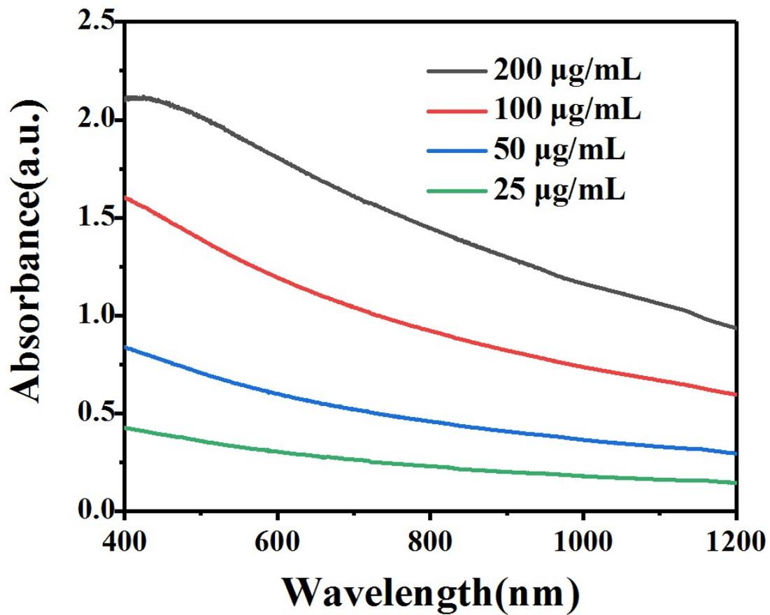
**Figure S15.** UV-vis-NIR absorption of the FeSA-HNCSB nanozyme with different concentrations.
