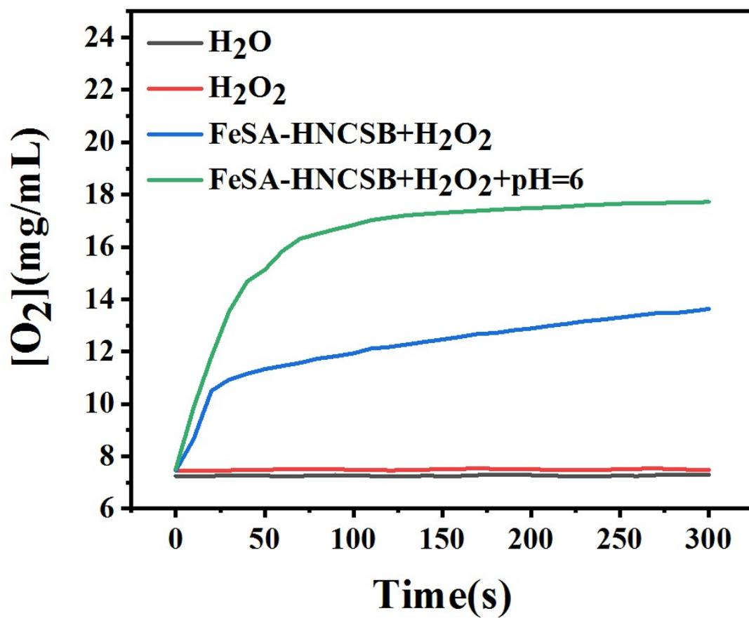
**Figure S12.** Concentration curves of dissolved oxygen in different experimental groups.  $100 \mu\text{g mL}^{-1}$  FeSA-HNCSB,  $0.1 \text{ mM H}_2\text{O}_2$ .
