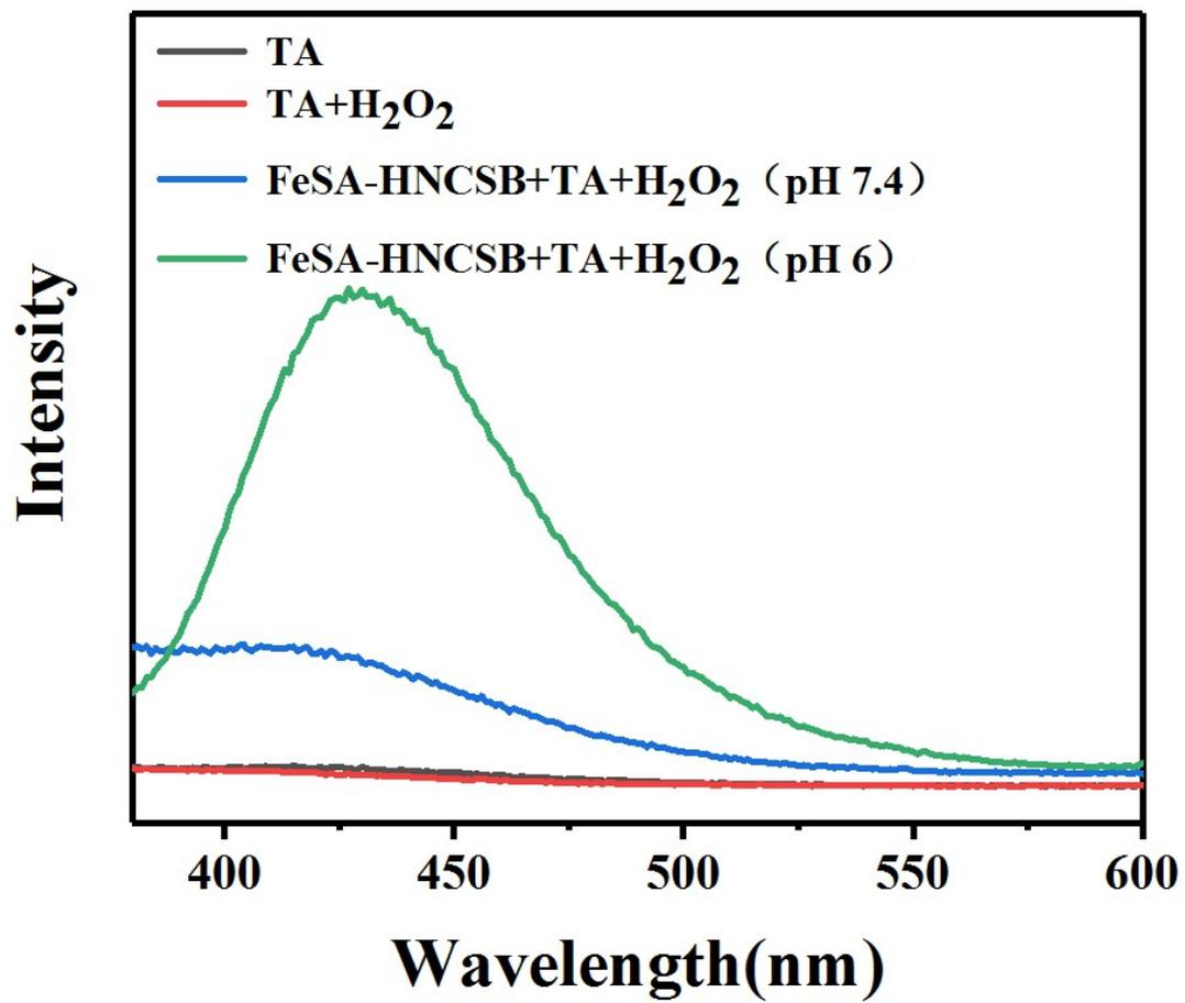
**Figure S14.** Fluorescence spectra of terephthalic acid representing the content of hydroxyl radical in different experimental groups.
