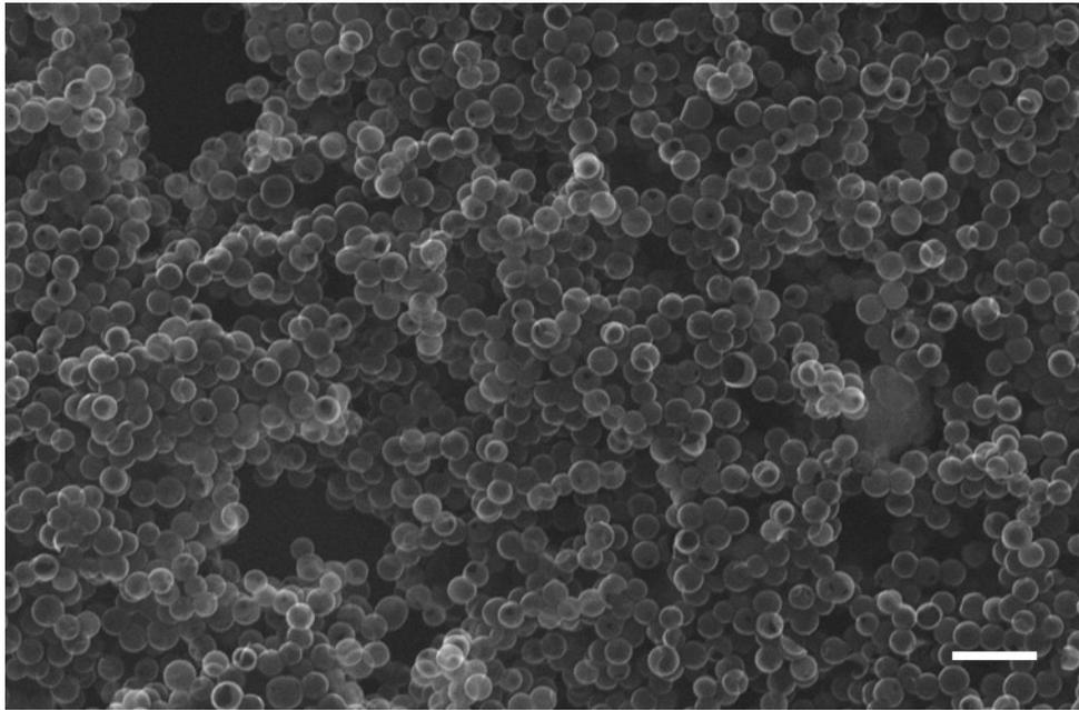
**Figure S3.** SEM image of FeSA-HNCS nanozyme. Scale bar=1  $\mu\text{m}$ .
