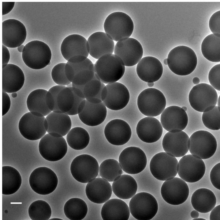
**Figure S1.** TEM image of SiO<sub>2</sub>, which exhibits uniform spherical with a diameter of about 250 nm. Scale bar=50 nm.
