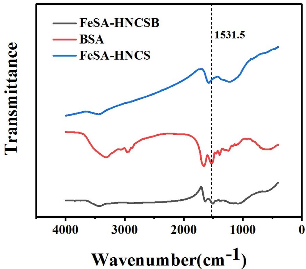
**Figure S10.** The Fourier transform infrared (FTIR) spectra of BSA, FeSA-HNCS, and FeSA-HNCSB.
