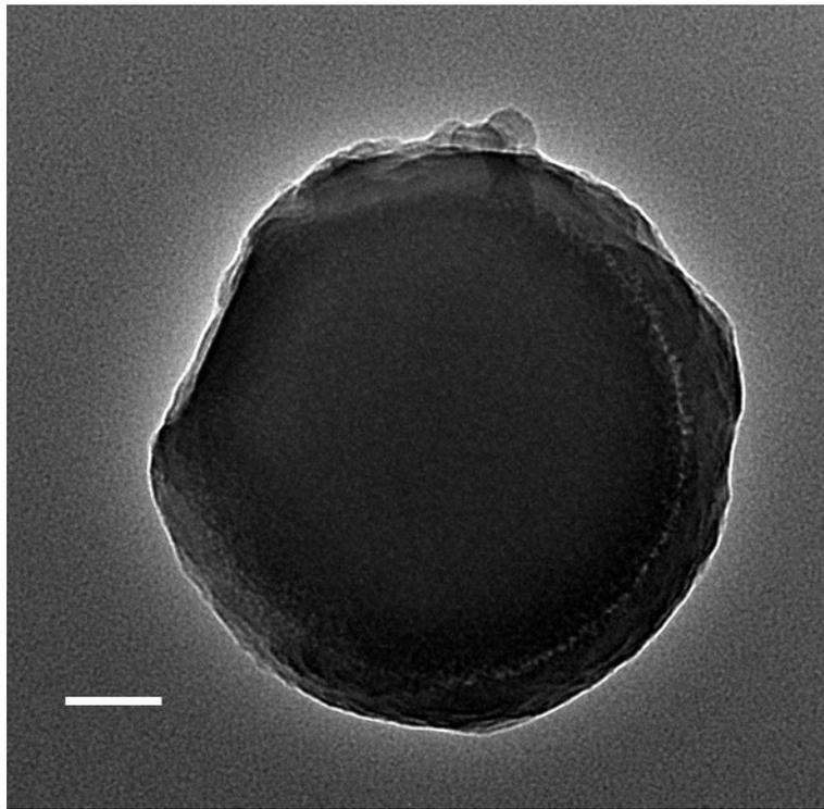
**Figure S2.** TEM image of SiO<sub>2</sub>@Fe-PDA , which exhibits uniform core-shell structure. Scale bar=50 nm.
