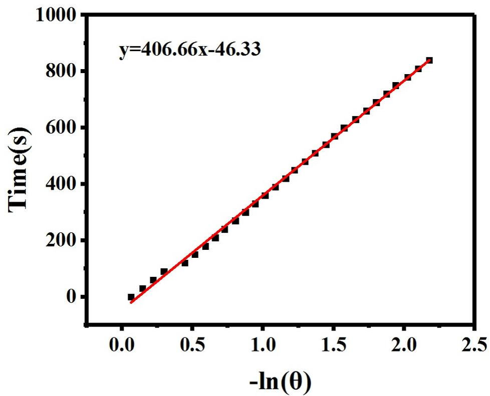
**Figure S17.** The linearity curves about time and  $-\ln\theta$  fitted from the temperature cooling process of FeSA-HNCSB nanozyme.
