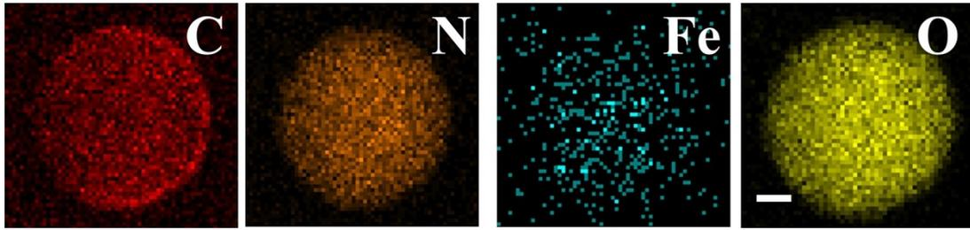
**Figure S4.** The EDS maps of C, N, Fe and O (scale bar 50 nm).
