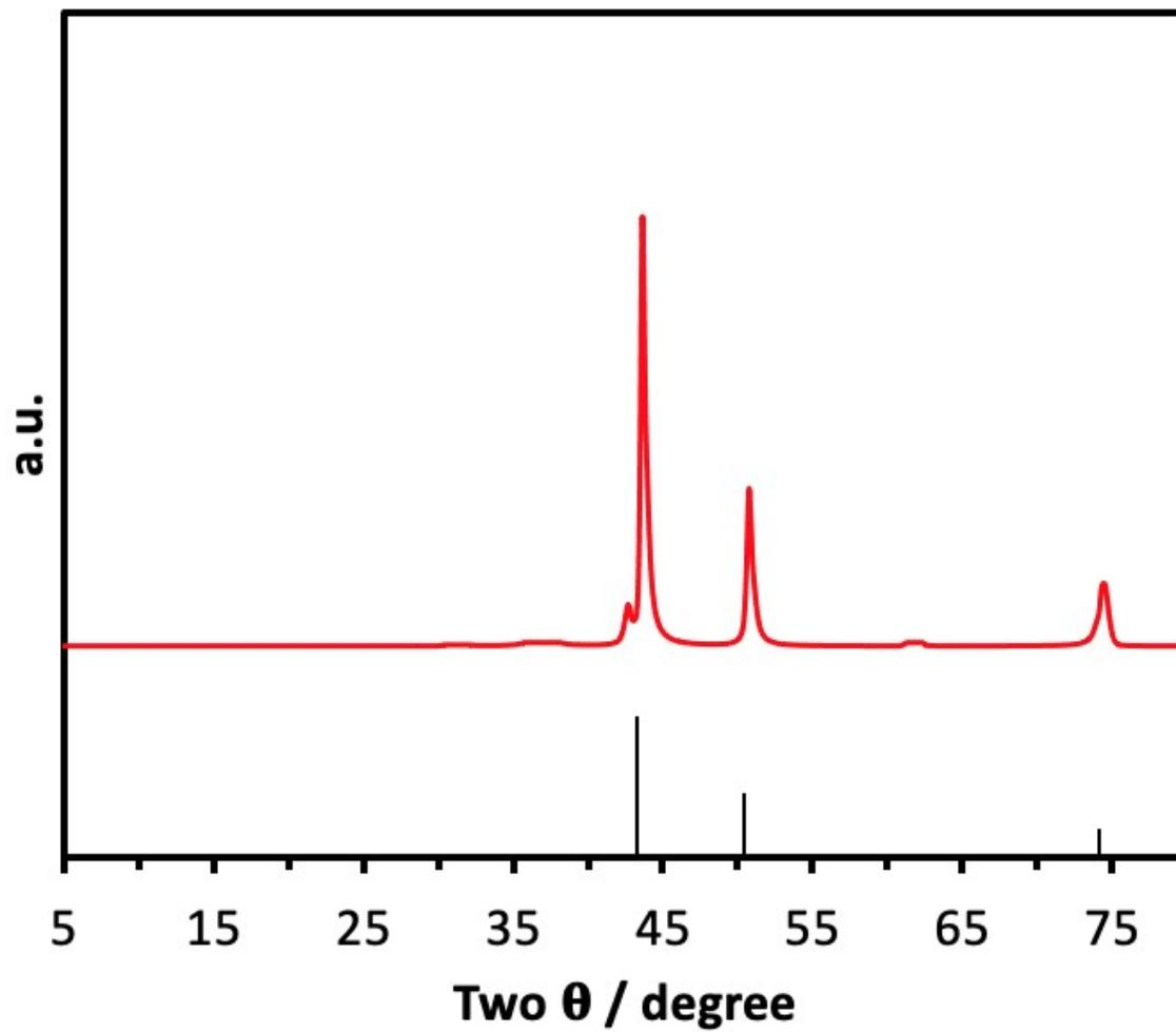
**Figure S3.** *Ex situ* XRD pattern of the fully discharged copper electrode in 16 m KF. The discharged electrode is confirmed to be copper (PDF#04-0836).
