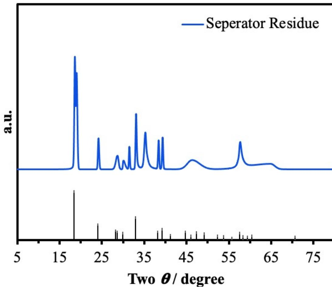
**Figure S4.** *Ex situ* XRD pattern of the separator residue. Contents on the surface of the separator were removed with a scalpel and confirmed to be monoclinic  $\text{CuF}_2$  (PDF #06-143).
