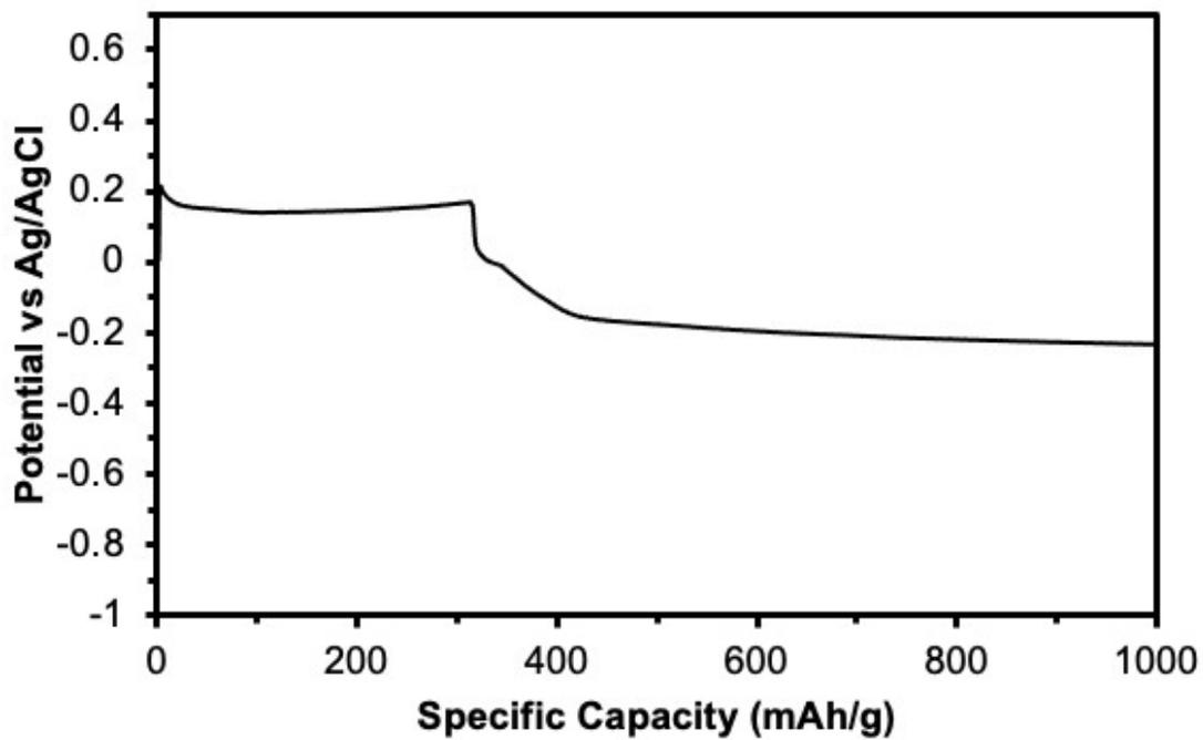
**Figure S1.** GCD potential profile for the 1<sup>st</sup> charge in 1 *m* KF at 500 mA/g. The cell failed before the discharge process starts.
