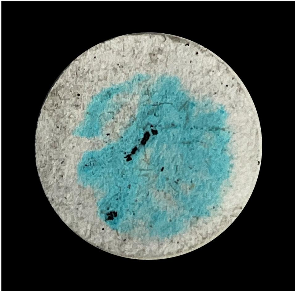
**Figure S2.** Image of the separator from a cycled cell after 300 cycles in 16 *m* KF. The separator was collected and dried/stored under vacuum.
