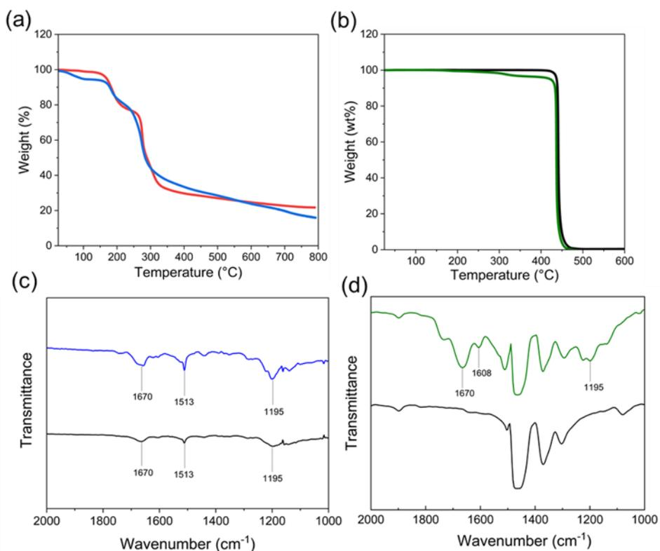
**Fig. S4** Physical characterization of the polymer films. (a) Thermogravimetric analysis of the peptide (blue) and peptide assemblies (red). (b) neat LDPE (black) and LDPE/peptide (green). (c) ATR-FTIR spectra of peptide assemblies before (blue) and after (black) freeze-drying and heating at 160 °C for 11 min. (d) FT-IR spectra of neat LDPE (black) and LDPE/peptide (green).
