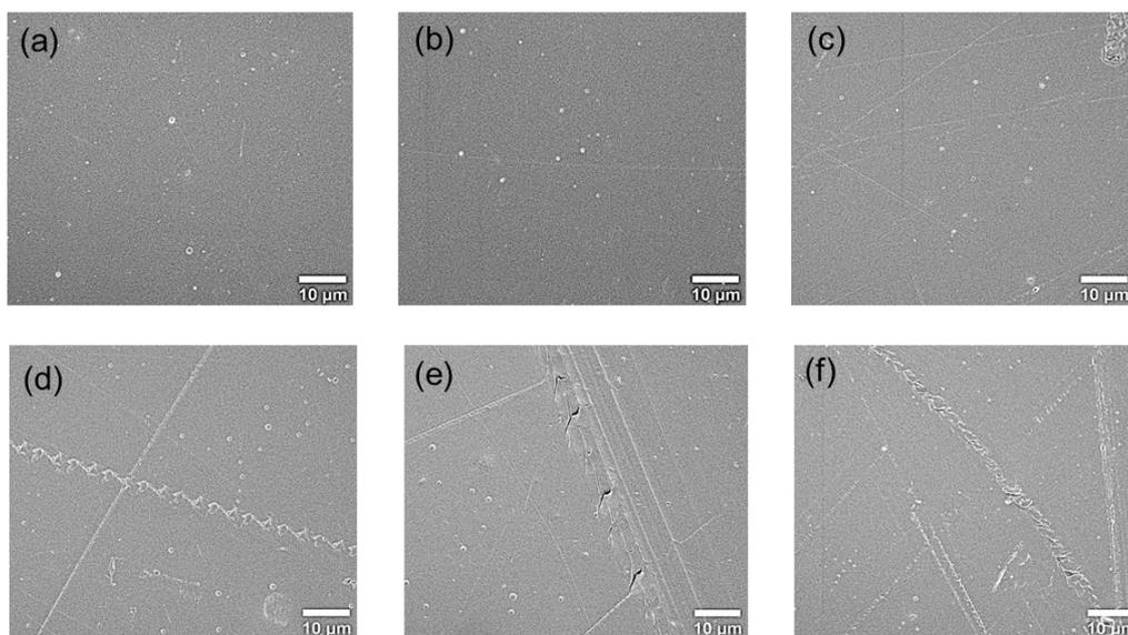
**Fig. S11** HR-SEM images of the LDPE/peptide films after exposure to different conditions. (a) immediate exposure to ethanol (b) 1h exposure to ethanol, (c) 24h exposure to ethanol, (d) immediate exposure to TDW after scratching, (e) 1h exposure to TDW after scratching, and (f) 1h exposure to TDW after scratching.
