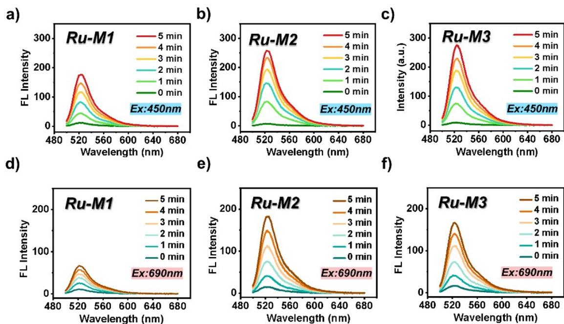
**Figure S 13.** ROS generation of a) **Ru-M1**; b) **Ru-M2**; c) **Ru-M3** illuminated by 450 nm laser ( $18.0 \text{ mW}\cdot\text{cm}^{-2}$ ) and d) **Ru-M1**; e) **Ru-M2**; f) **Ru-M3** illuminated by 690 nm laser ( $0.9 \text{ W}\cdot\text{cm}^{-2}$ ) using  $\text{H}_2\text{-DCFH}$  as an indicator.
