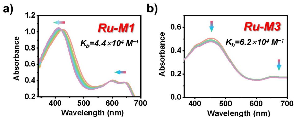
**Figure S17.** UV-vis spectra of **Ru-M1** a) and **Ru-M3** b) upon addition of ctDNA (0–0.1 mM) in 5 mM Tris·HCl buffer solution (pH = 7.2). The arrows show the change of absorbance upon the addition of ctDNA.
