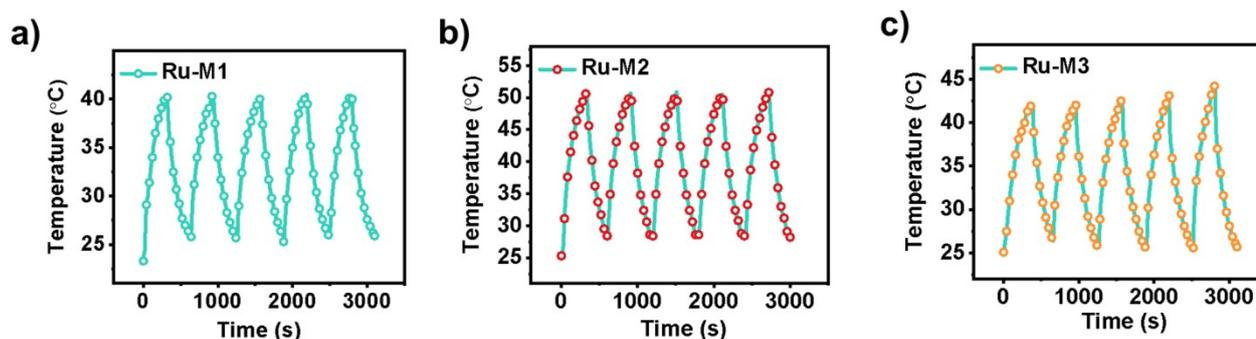
**Figure S16.** a) Photothermal heating/nature cooling cycles of **Ru-M1** ( $20 \mu\text{M}$ ) under 690 nm laser irradiation ( $0.9 \text{ W}\cdot\text{cm}^{-2}$ ); b) Photothermal heating/nature cooling cycles of **Ru-M2** ( $20 \mu\text{M}$ ) under 690 nm laser irradiation ( $0.9 \text{ W}\cdot\text{cm}^{-2}$ ); c) Photothermal heating/nature cooling cycles of **Ru-M3** ( $20 \mu\text{M}$ ) under 690 nm laser irradiation ( $0.9 \text{ W}\cdot\text{cm}^{-2}$ ).
