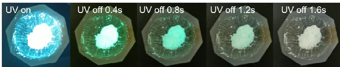
Figure S1. Photographs of ABP-MTPPC-0.1% powder in a mortar showing intense afterglow under daylight.
