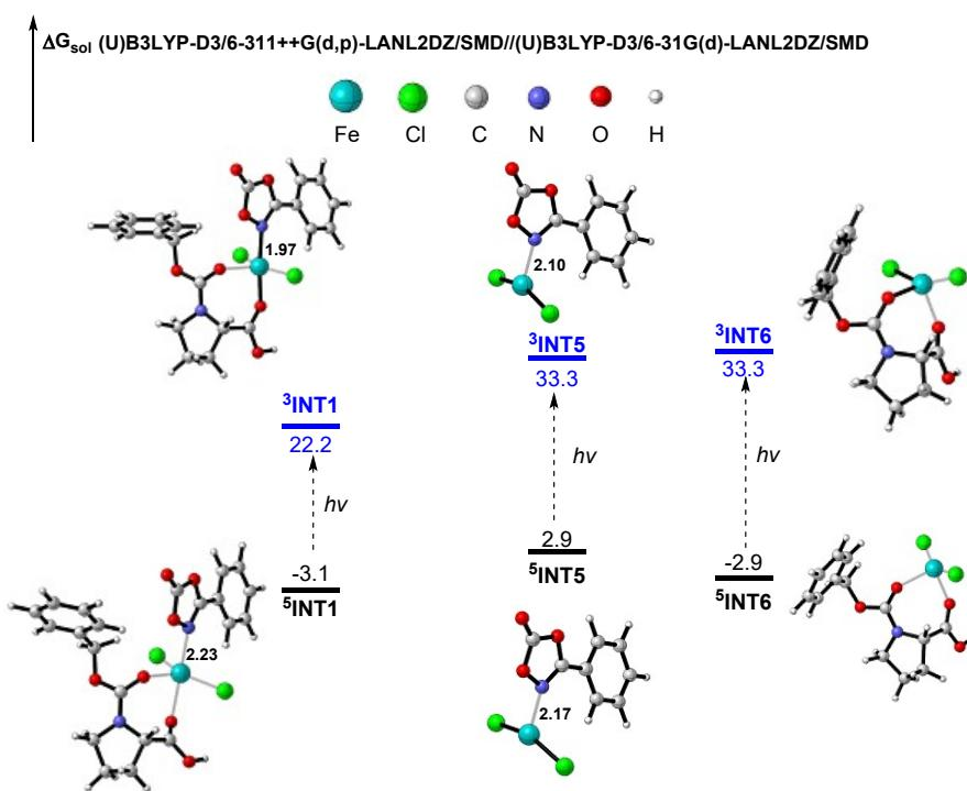
**Fig. S3** Energy profiles (in kcal/mol) for different coordination forms of the iron catalyst with  $\alpha$ -amino acids and dioxazolones. Bond lengths are shown in Å.
