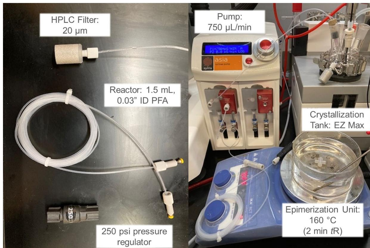
**Figure S2:** Reaction setup for Resolution of MRTX1719.
