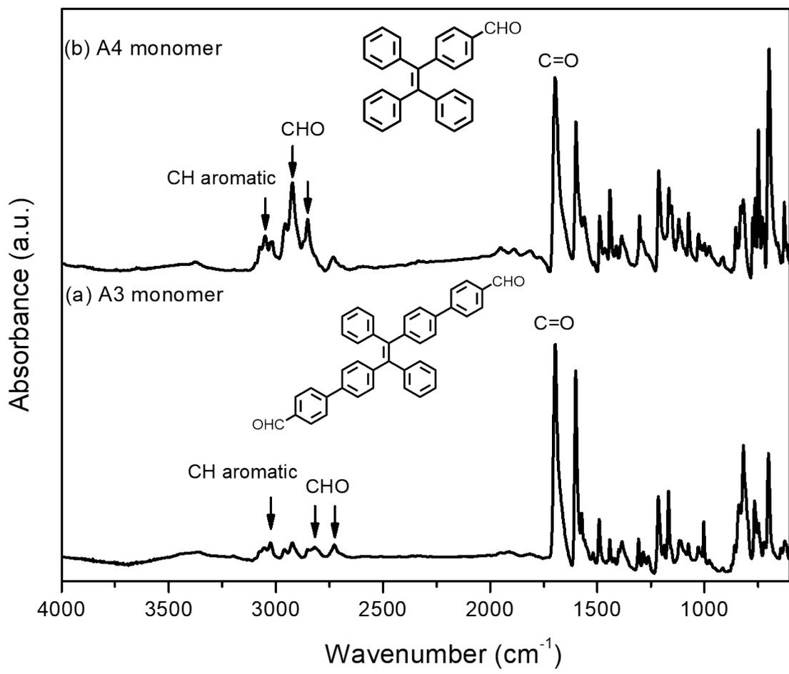
**Figure S3.** FT-IR spectra of (a) A3 and (b) A4 monomers.
