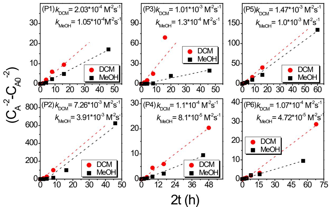
**Figure S6.** Kinetic analysis of P-MCPs in various solvents with the approach of 3<sup>rd</sup>-order reactions.
