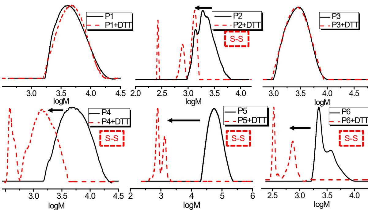
**Figure S11.** GPC traces of P1–P6 before (solid curves) and after (dash curves) DTT cleavages
