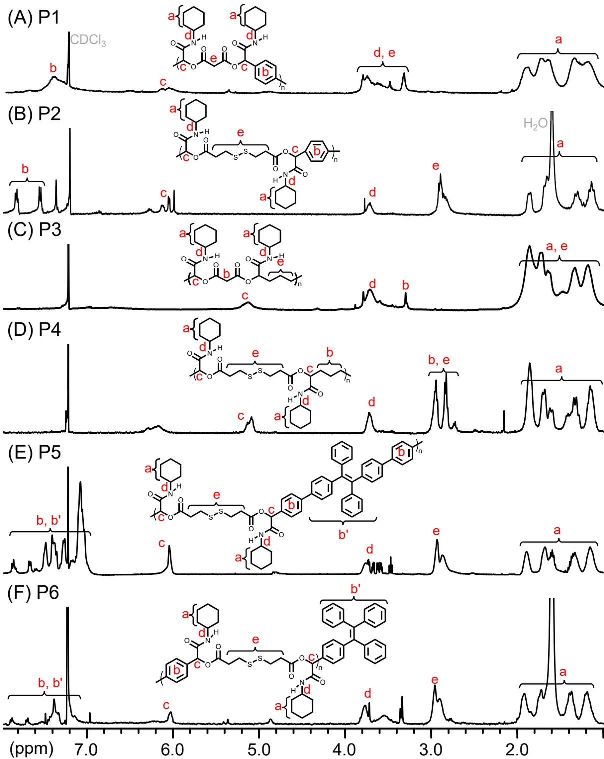
**Figure S8.**  $^1\text{H}$  NMR (400 MHz,  $\text{CDCl}_3$ ) spectra of (A–F) P1–P6 functional PCEs.
