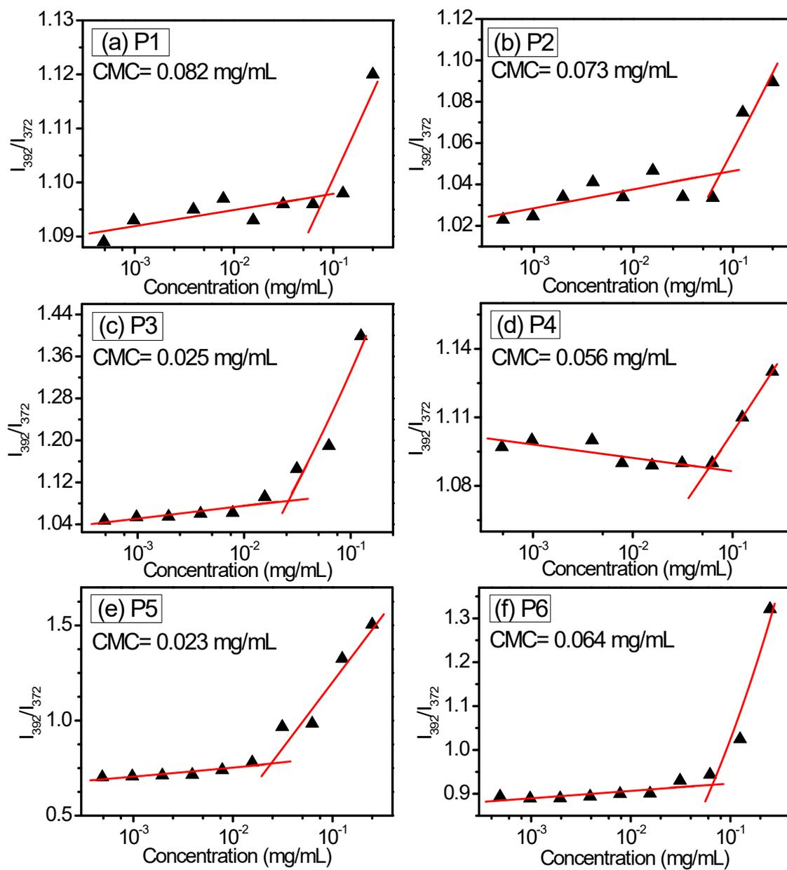
**Figure S9.** CMC plots of (a–f) P1–P6 traced by FL spectrometer.
