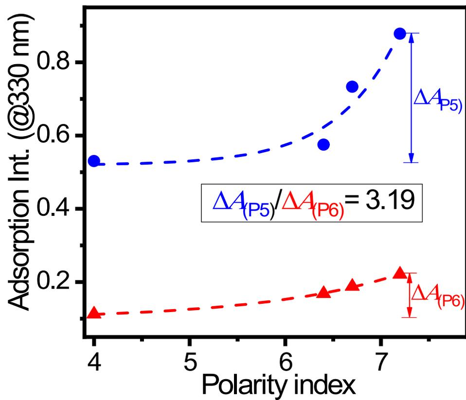
**Figure S16.** Relative trends of UV–Vis adsorption intensity variations ( $\Delta A$ ) at 330 nm vs polarity index of solvents of (a) P5 and (b) P6 estimated from UV–Vis spectra (i.e., **Fig. S15**).
