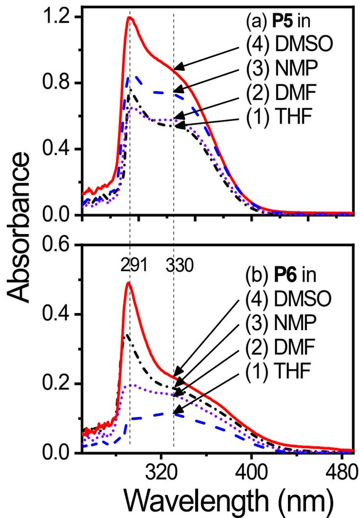
**Figure S15.** UV-Vis spectra of (a) P5 and (b) P6 in different solvents: (1) THF, (2) DMF, (3) NMP, and (4) DMSO.
