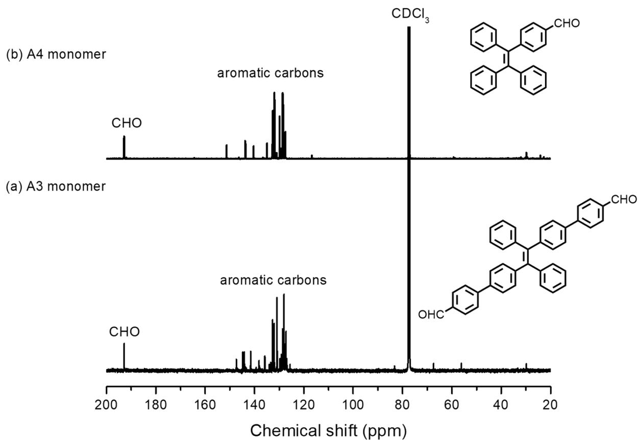
**Figure S2.**  $^{13}\text{C}$  NMR (400 MHz,  $\text{CDCl}_3$ ) spectra of (a) A3 and (b) A4 monomers.
