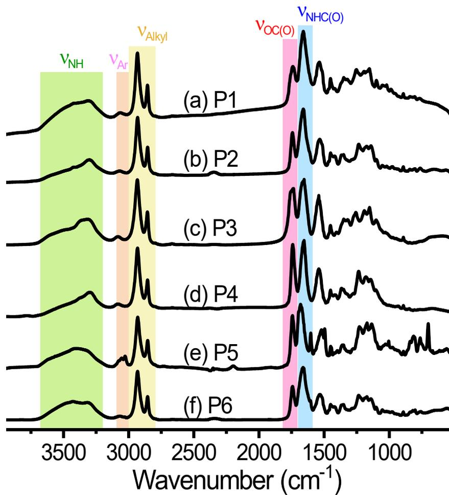
**Figure S7.** FT-IR spectra (3900–400 cm<sup>-1</sup>) of (a–f) P1–P6 functional PCEs.
