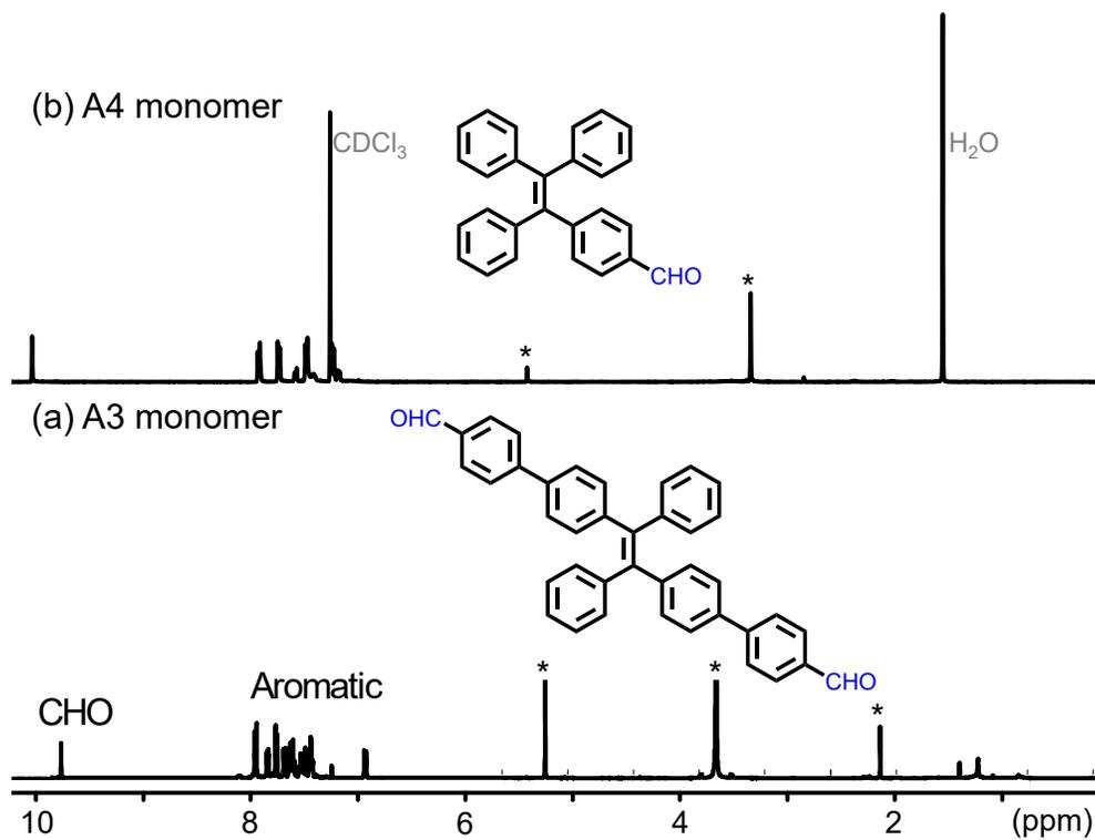
**Figure S1.** <sup>1</sup>H NMR (400 MHz, CDCl<sub>3</sub>) spectra of (a) A3 and (b) A4 monomers (\*: solvent peaks).
