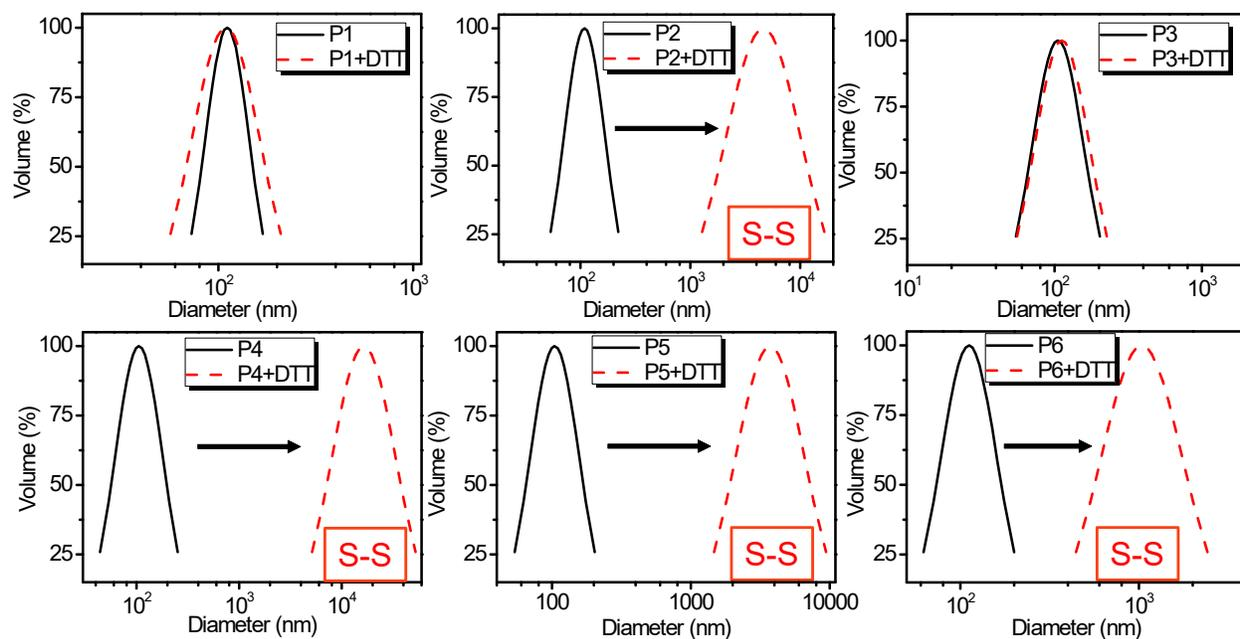
**Figure S12.** DLS differences of P1–P6 before and after DTT cleavages (S-S: containing disulfide linkages).
