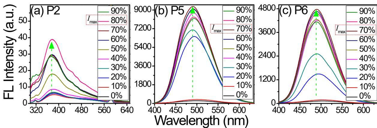
**Figure S17.** FL spectra of (a) P2 (400 V), (b) P5 (250 V), and (c) P6 (400 V) with various water vol.% in water and DMSO mixtures ( $\lambda_{\text{ex}} = 330 \text{ nm}$ ; V: voltage).
