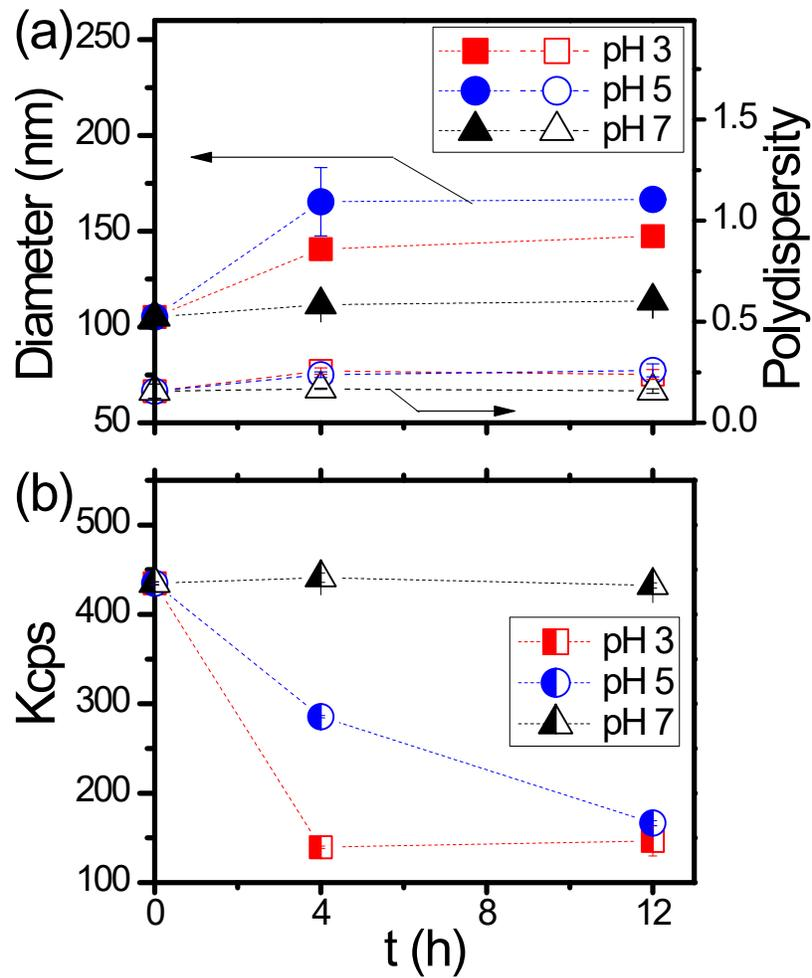
**Figure S13.** Micelle stabilities in different aqueous environments (i.e., pH = 3, 5, and 7 in 12 h at ambient) of P1–P6 measured by DLS.
