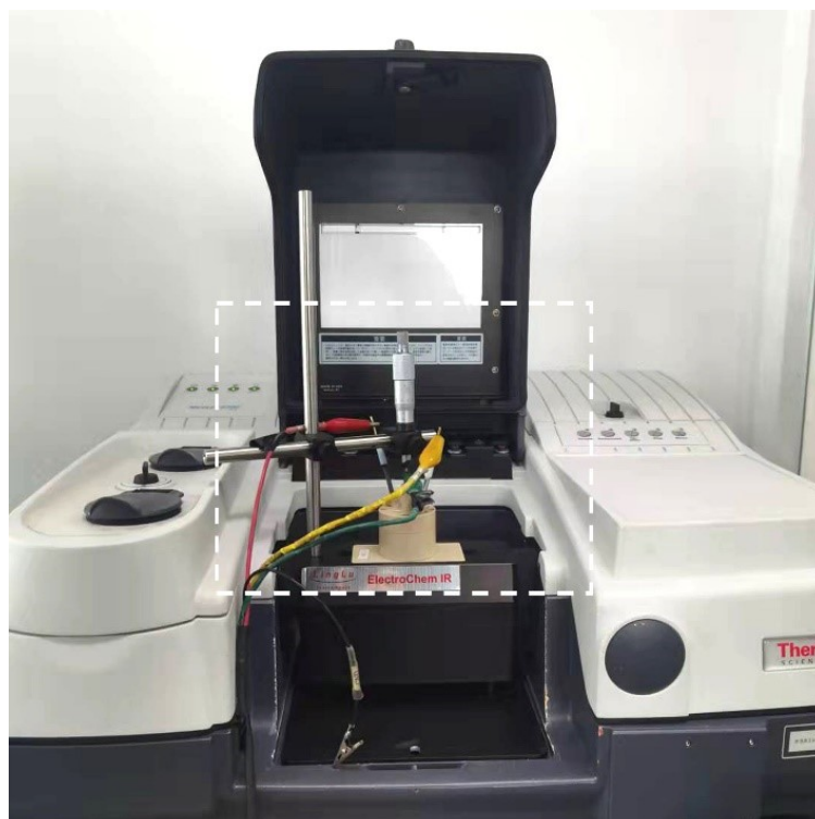
Fig. S9 Digital photo of in-situ FTIR system combined with electrochemical measurement.
