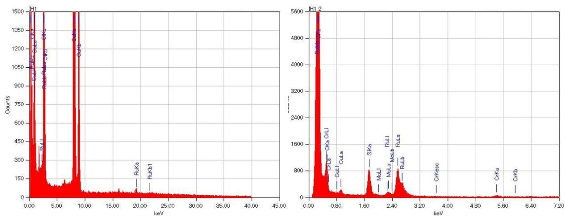
**Fig. S8.** Energy-dispersive X-ray spectroscopic analysis of Ru peaks
