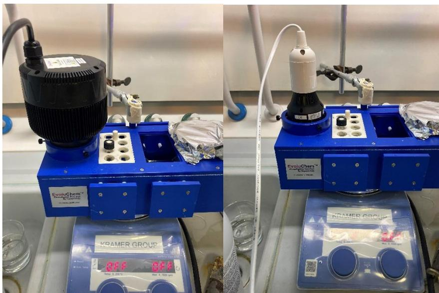
**Figure S1.** Hepatochem photoreactor. Left: 365 nm setup. Right: 425 nm setup.
