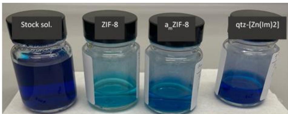
Figure S20: Photograph of methylene blue solutions after 48 hours of stirring with ZIF-8,  $a_m$ ZIF-8 and  $qtz$ -[Zn(lm)<sub>2</sub>], followed by filtering. The starting stock solution is presented for reference.
