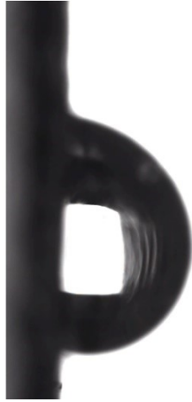
Fig. S8. Due to the large contact angle hysteresis of the pristine composite surface, a droplet and bubble cannot slide on the surface even if the surface was tilted at 90^\circ .
