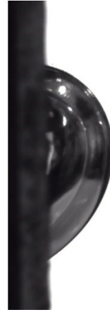
Fig. S8. Due to the large contact angle hysteresis of the pristine composite surface, a droplet and bubble cannot slide on the surface even if the surface was tilted at 90^\circ .
