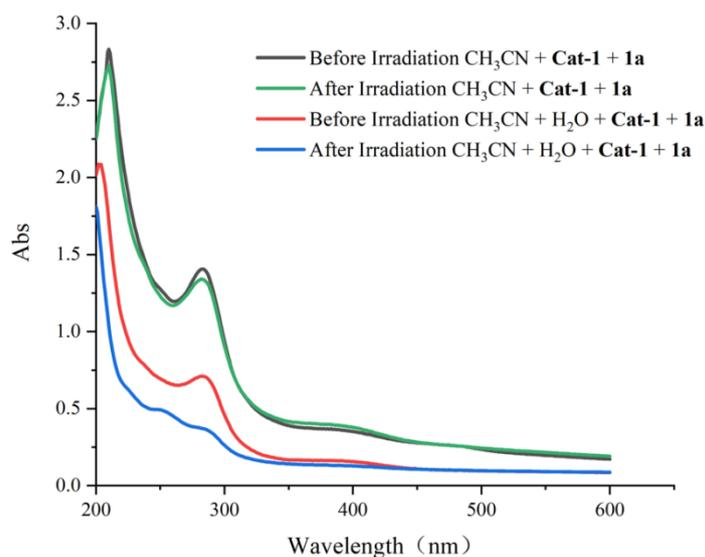
**Figure S2.** UV-vis absorption spectra for the mixture of **Cat-1** and **1a** in CH<sub>3</sub>CN and CH<sub>3</sub>CN/H<sub>2</sub>O before and after blue LED irradiation (455 nm).
