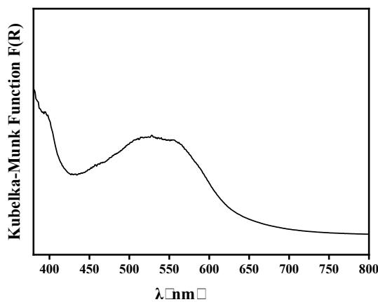
**Fig. S7.** Ultraviolet-visible diffuse reflectance spectroscopy of cage **1** recorded at room temperature.
