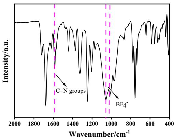
**Fig. S5** FT-IR of cage **1** recorded at room temperature.
