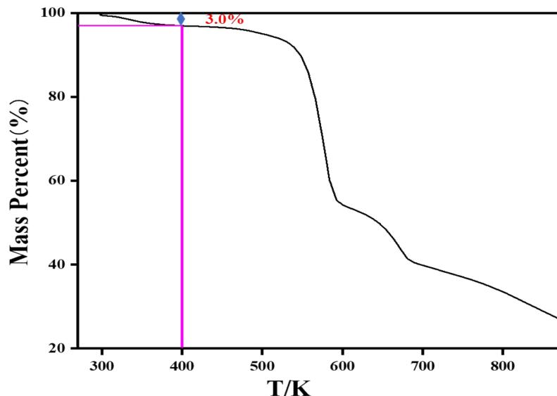
**Fig. S8.** TGA curve of cage **1** and the abscissa of the magenta line is 400 K. The mass loss of c.a. 3.0% from room temperature to 400 K, which is attributed to the release of 7 water molecules, matching well elemental analysis result (3.2 %).
