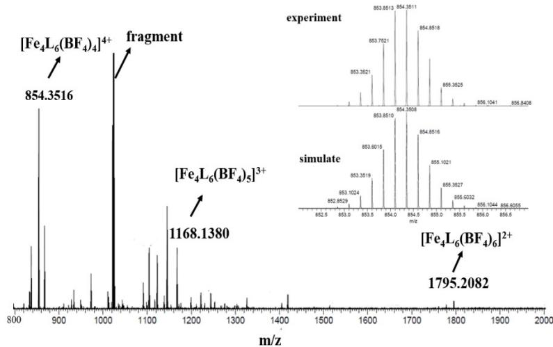
ESI-HRMS spectrum of cage 1. The inset shows the isotope pattern for  $[\text{Fe}_4\text{L}_6(\text{BF}_4)_4]^{4+}$  with the simulated distribution.
