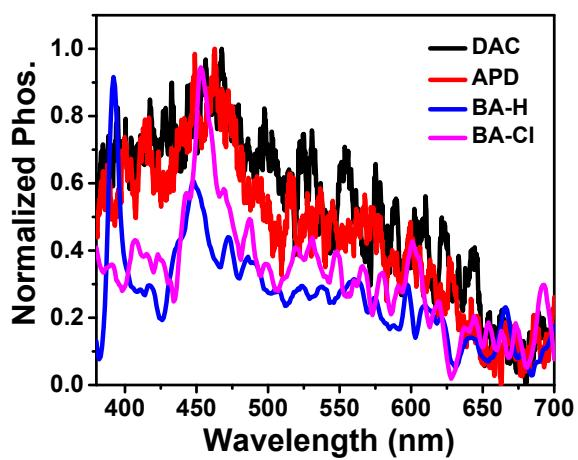
**Figure S6.** Delayed emission spectra of four hosts in solid state. (Delay time: 0.5 ms; Ex.: 380 nm).
