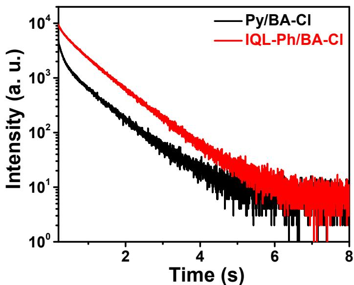
**Figure S19.** Phosphorescence decay curves of Py/BA-Cl and IQL-Ph/BA-Cl.
