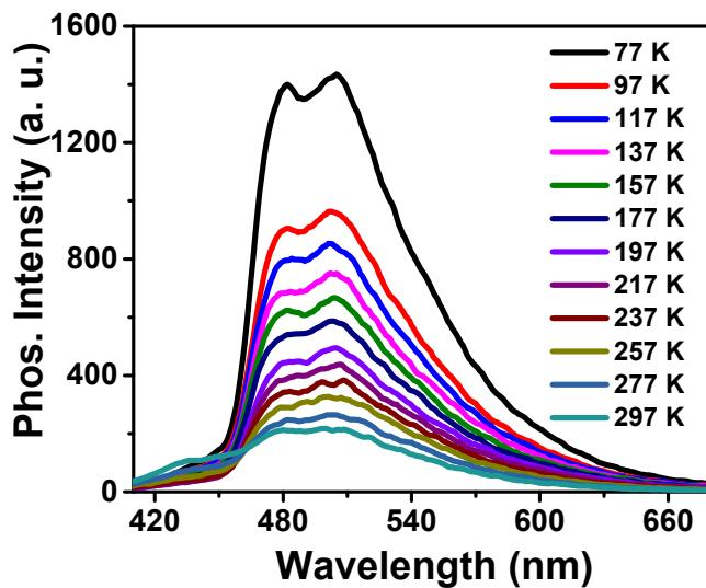
**Figure S9.** Delayed emission intensity of **Mb/BA-Cl** at different temperatures.
