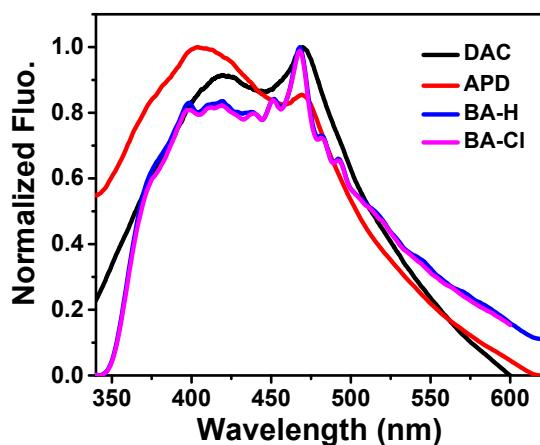
**Figure S5.** Fluorescence emission spectra of four hosts in solid state. (Ex.: 330 nm).
