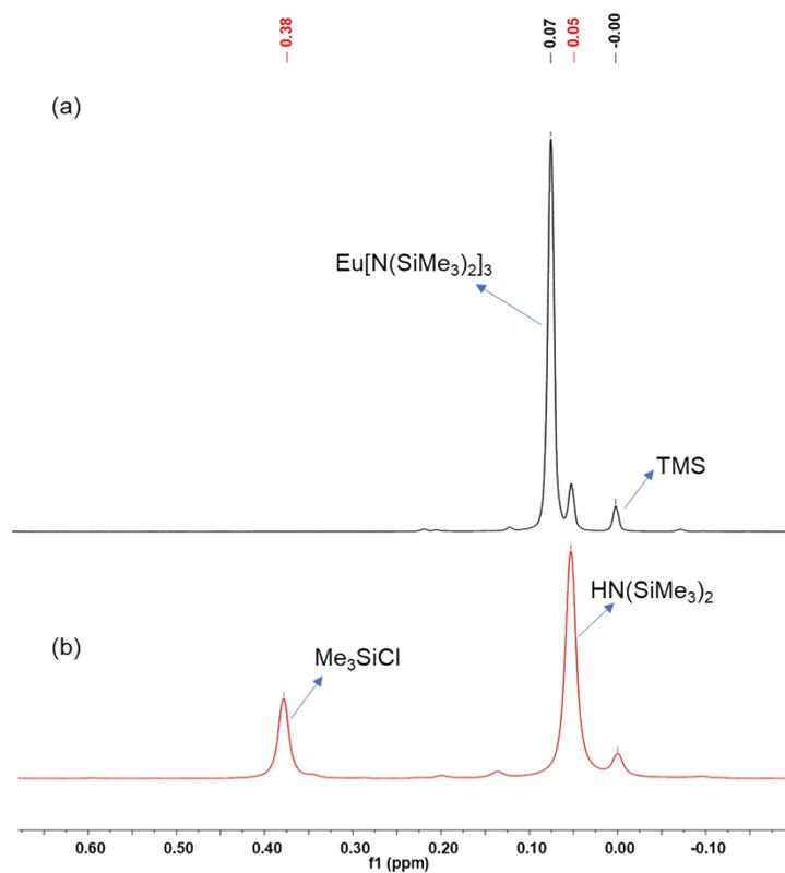
**Fig. S2.** (a)  $^1\text{H}$  NMR spectrum of  $\text{Eu}[\text{N}(\text{SiMe}_3)_2]_3$  in  $n\text{-hexane-}d_{14}$ . (b)  $^1\text{H}$  NMR spectrum of the reaction of  $\text{Eu}[\text{N}(\text{SiMe}_3)_2]_3$  with  $\text{CHCl}_3$  (1:1) at room temperature in  $n\text{-hexane-}d_{14}$ .
