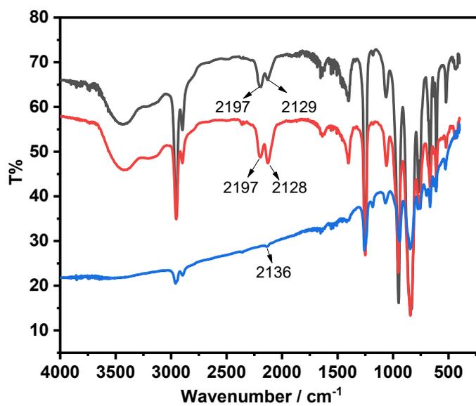
**Fig. S7.** FTIR spectra of complex **1** (black), **2** (red) and **3** (blue).
