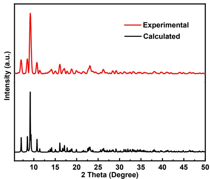
**Fig. S5.** Experimental and calculated PXRd patterns for  $[\text{Sm}\{\text{N}(\text{SiMe}_3)_2\}_2(\mu\text{-Cl})(\text{NCSiMe}_3)_2]$ .
