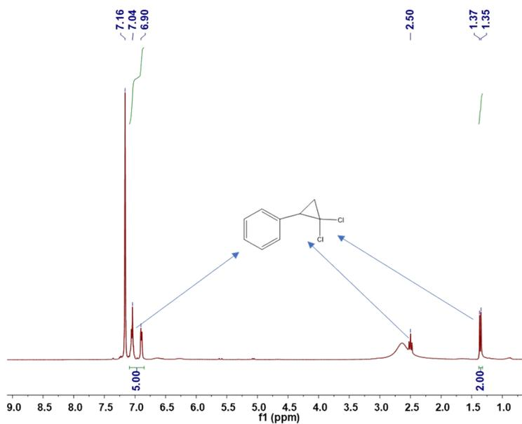
**Fig. S1.**  $^1\text{H}$  NMR ( $\text{C}_6\text{D}_6$ ) spectrum of the reaction products of  $\text{Eu}[\text{N}(\text{SiMe}_3)_2]_3$  with styrene and  $\text{CDCl}_3$  (1:1:1) at room temperature in n-hexane. The reaction mixture was filtered and the solvent was removed before the reaction products were dissolved in  $\text{C}_6\text{D}_6$ .
