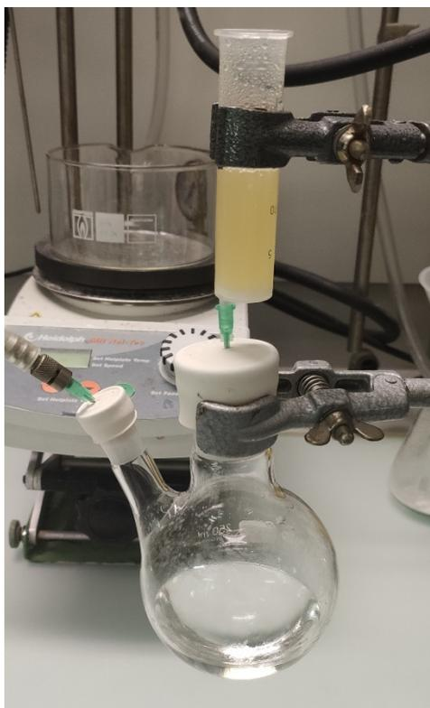
**Fig. S8.** Reaction set-up for the resin loading using a syringe equipped with a frit and a flow of nitrogen.
