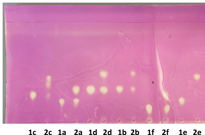
Figure S4. GOase F 2 Substrate screening using thin layer chromatography (TLC, silica). MeCN/0.1% formic acid 99:1. In all cases, the oxidised products 2a-f appear as the top spot, with higher R f value than the starting materials 1a-f .
