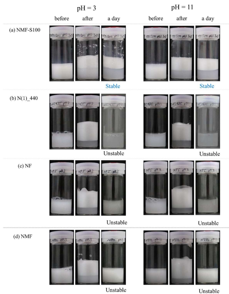
Figure S6. Foaming test and characterization of foam stability with various types of microgels, NC microgels, and solid microspheres under different pH conditions (pH = 3 or 11). All foams were prepared by mixing 1 wt.% colloid dispersion at 10,000 rpm for 1 min at room temperature (25 °C). The foams were stored at room temperature for 1 day. The time-dependence of the foam diameter was also characterized using an optical microscope. Foams stabilized by NC microgels (NFM-S100) showed high storage stability regardless of the pH value of the solution.
