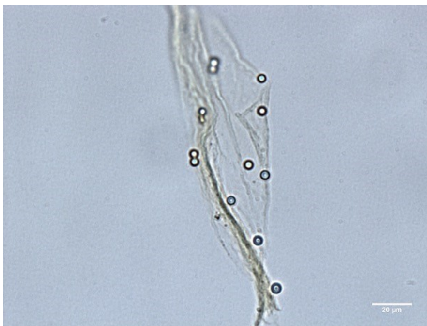
Figure S14: Figure showing negatively charged microparticles adhering to the surface of PEI-FITC films.
