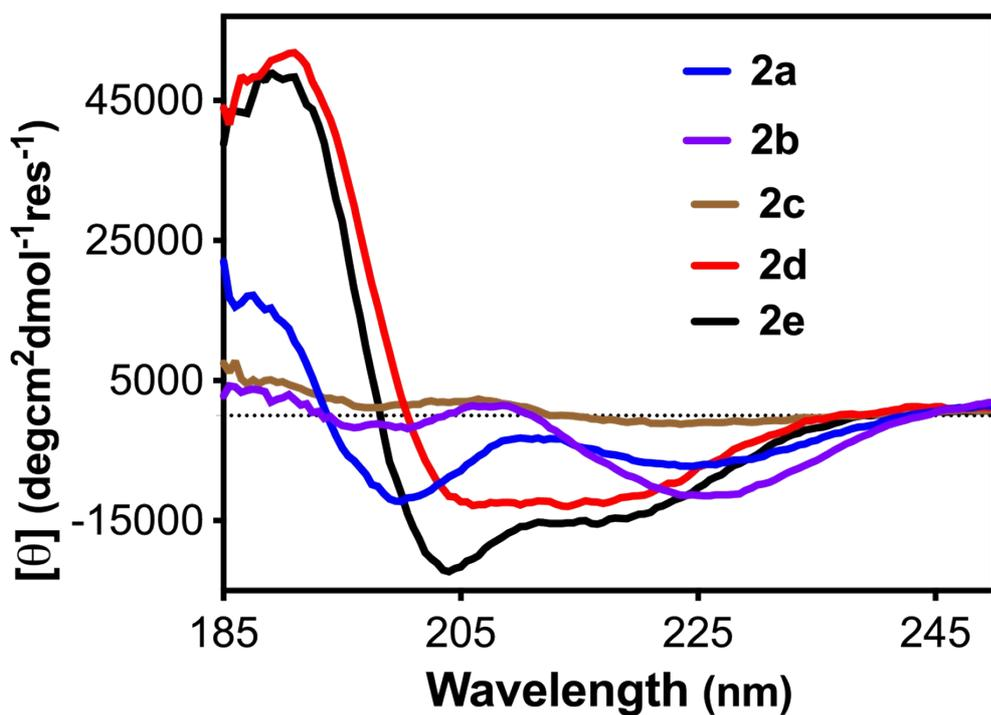
**Figure S7.** Raw CD spectra for N-methylated peptides **2a-e** (100  $\mu$ M) in phosphate buffer (10mM, pH 7.4, 298K).
