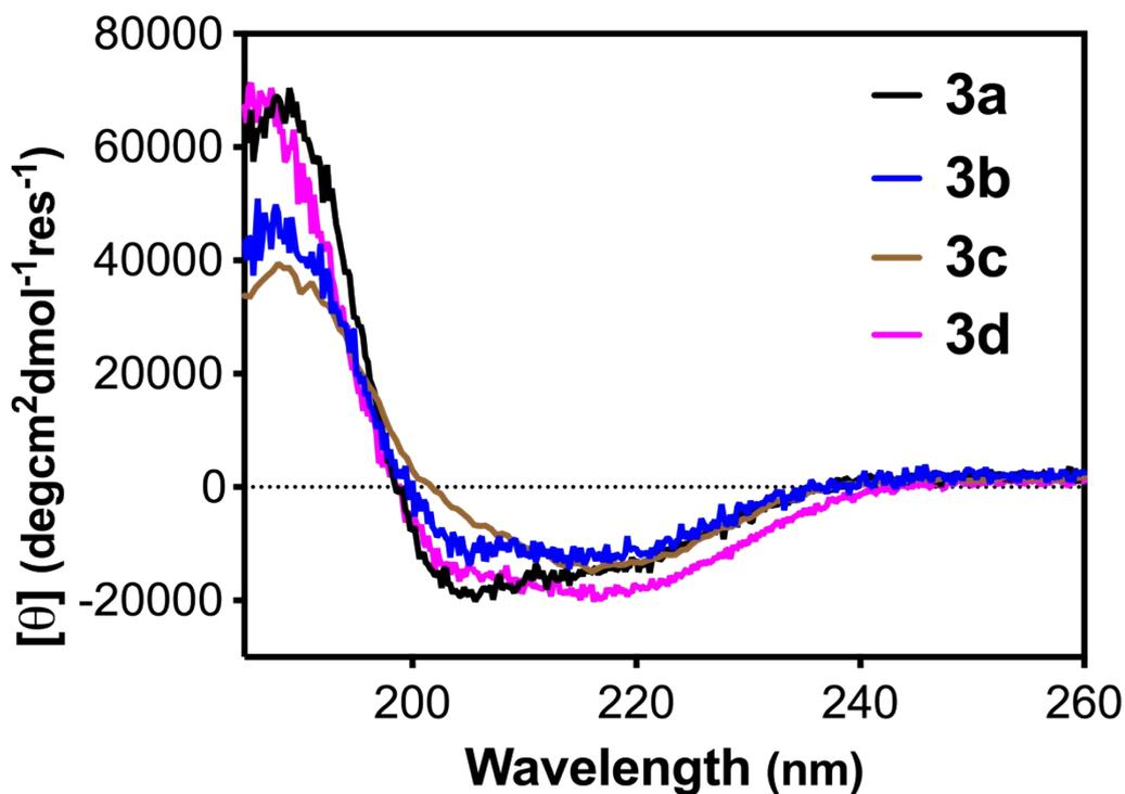
**Figure S8.** Raw CD spectra for monoesters **3a-c** (100  $\mu$ M) in phosphate buffer (10 mM, pH 7.4, 298K) and triester **3d** (250  $\mu$ M) in 70%  $\text{CD}_3\text{CN}$  in water for solubility.
