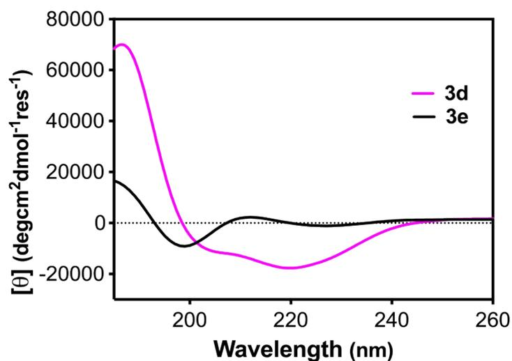
**Figure S5.** CD spectra for esters **3d** (250  $\mu$ M 70%  $\text{CD}_3\text{CN}$  for solubility) and **3e** (100  $\mu$ M) in phosphate buffer (10mM, pH 7.4, 298K). Indicates no helical structure in **3e**.
