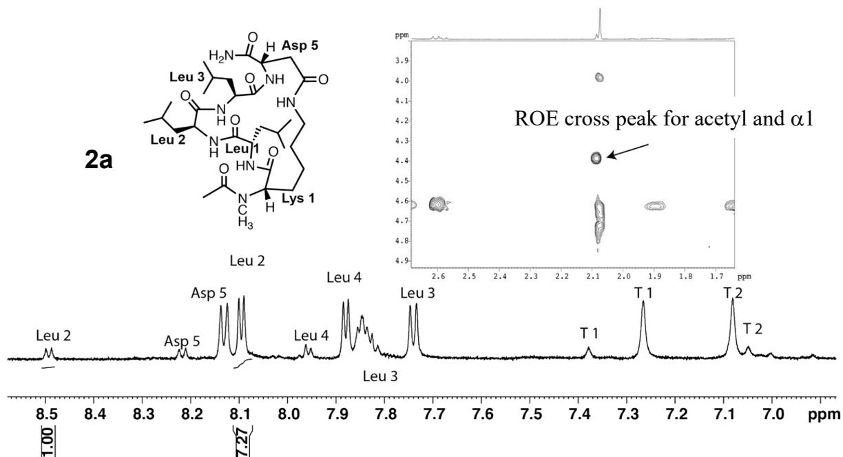
**Figure S1.**  $^1\text{H}$  NMR amide chemical shift region for **2a** and ROE cross peak between acetyl cap and  $\alpha 1$  (Lys H $\alpha$ ) in  $\text{H}_2\text{O}:\text{D}_2\text{O}$  (9:1).
