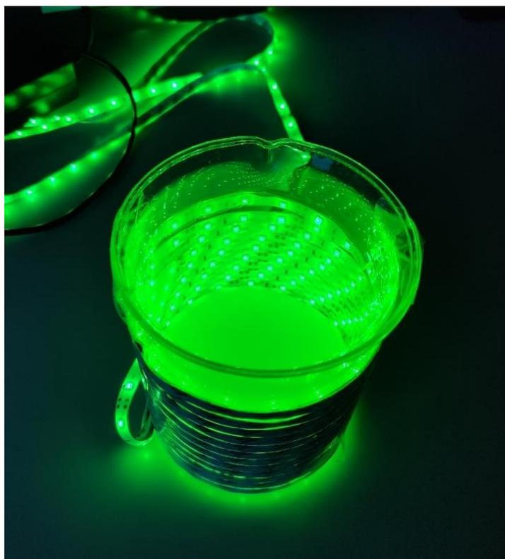
**Figure S 1** Home-built photoreactor for photo catalytic experiments.
