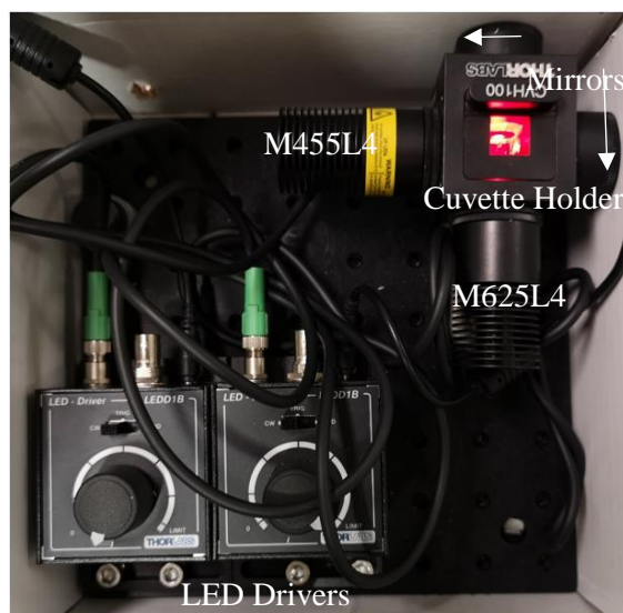
Figure S48. Apparatus for photo-irradiating small liquid samples
