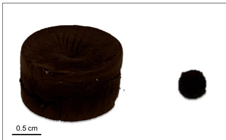
Figure S10. Photographs of GDY aerogel monolith (left) and GDY xerogel monolith (right). The GDY xerogel was obtained by open-atmosphere drying. The volume of GDY aerogel is 2.035 \text{ cm}^3 (1.8 cm of diameter and 0.8 cm of height), while the volume of GDY xerogel is 0.039 \text{ cm}^3 (0.5 cm of diameter and 0.2 cm of height).
