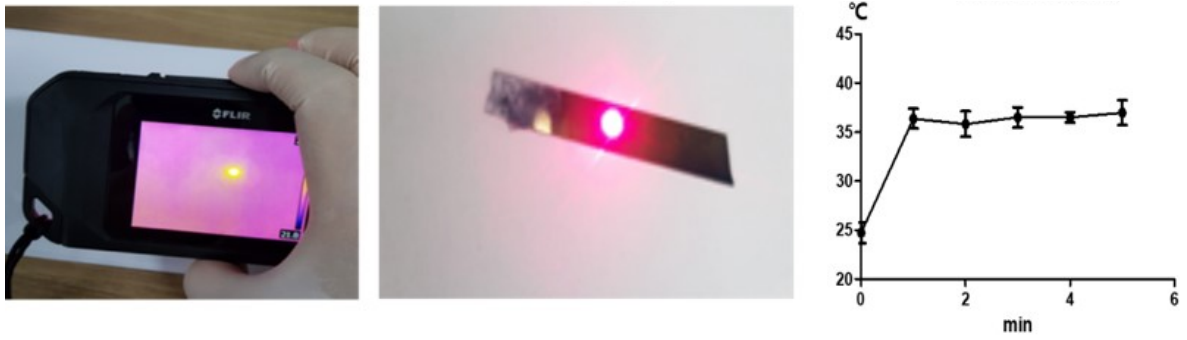
Fig. S4. Photothermal temperature rises of AuNRs assembled on glass plates irradiated with 30 mW, 671 nm laser.
