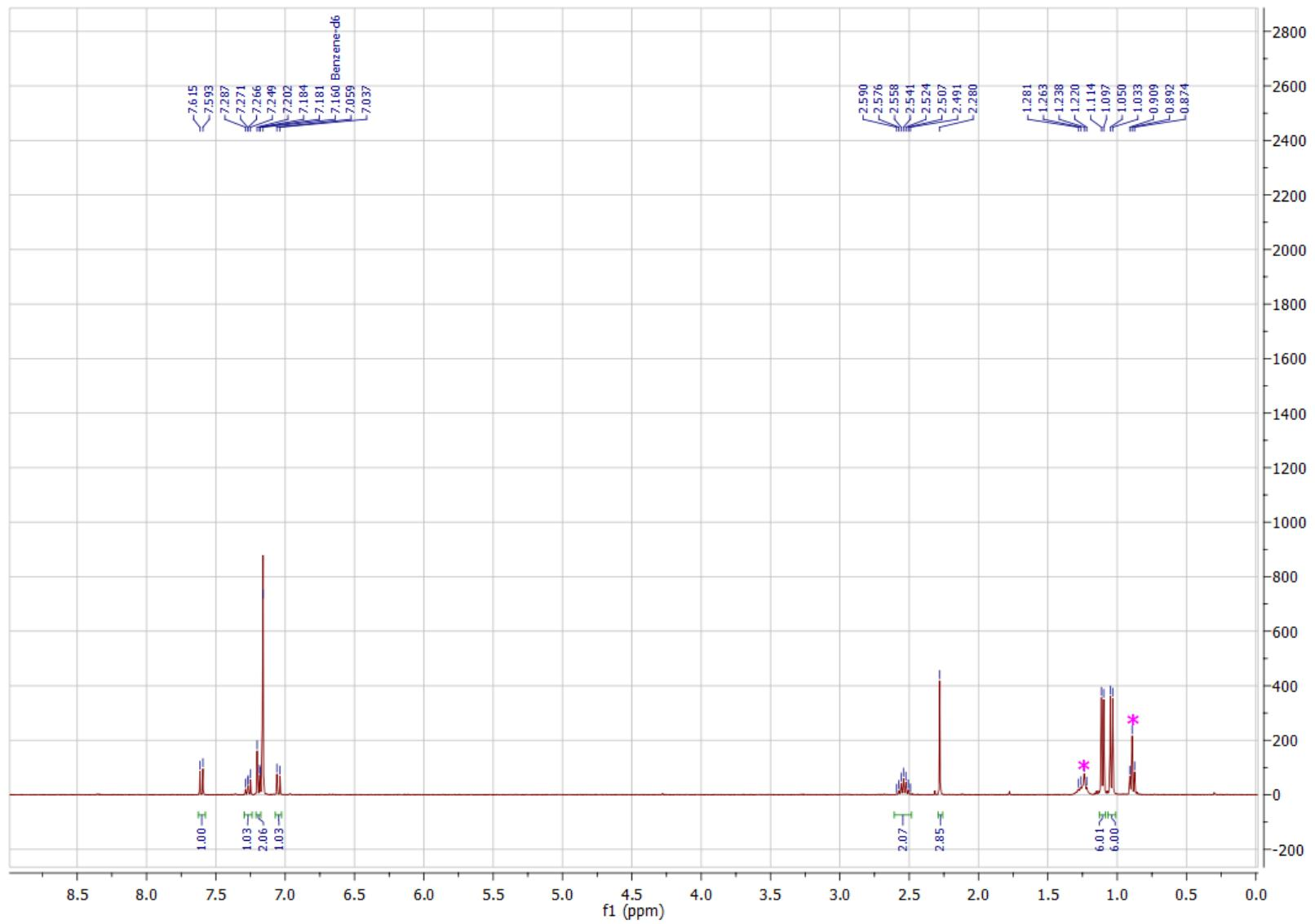
**Fig. S5** <sup>1</sup>H NMR spectrum of NDI-Ge<sub>2</sub> **3** in C<sub>6</sub>D<sub>6</sub>. (Hexane residue is denoted by pink stars)
